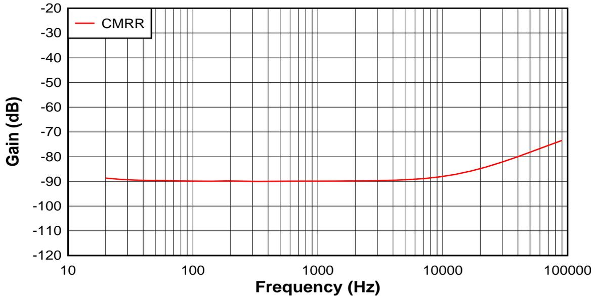
Figure 6. Common-Mode Rejection Ratio (CMRR) Measurement
