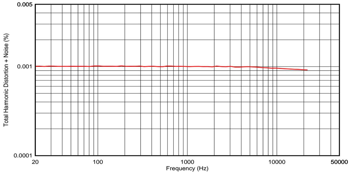
**Figure 8. THD+N vs. Frequency Measurement with  $1 V_{RMS}$  Output
