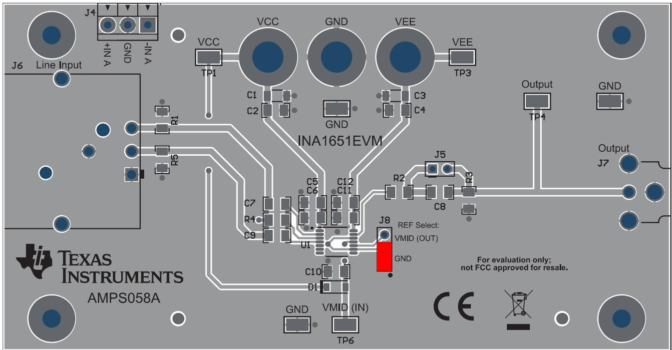
Figure 5. J8 Connection for Dual Supply Operation
