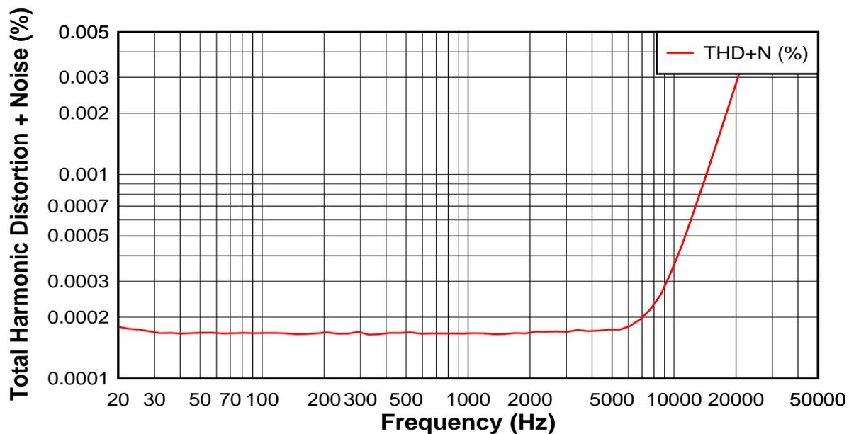
**Figure 9. THD+N vs. Frequency Measurement With  $10 V_{RMS}$  Output
