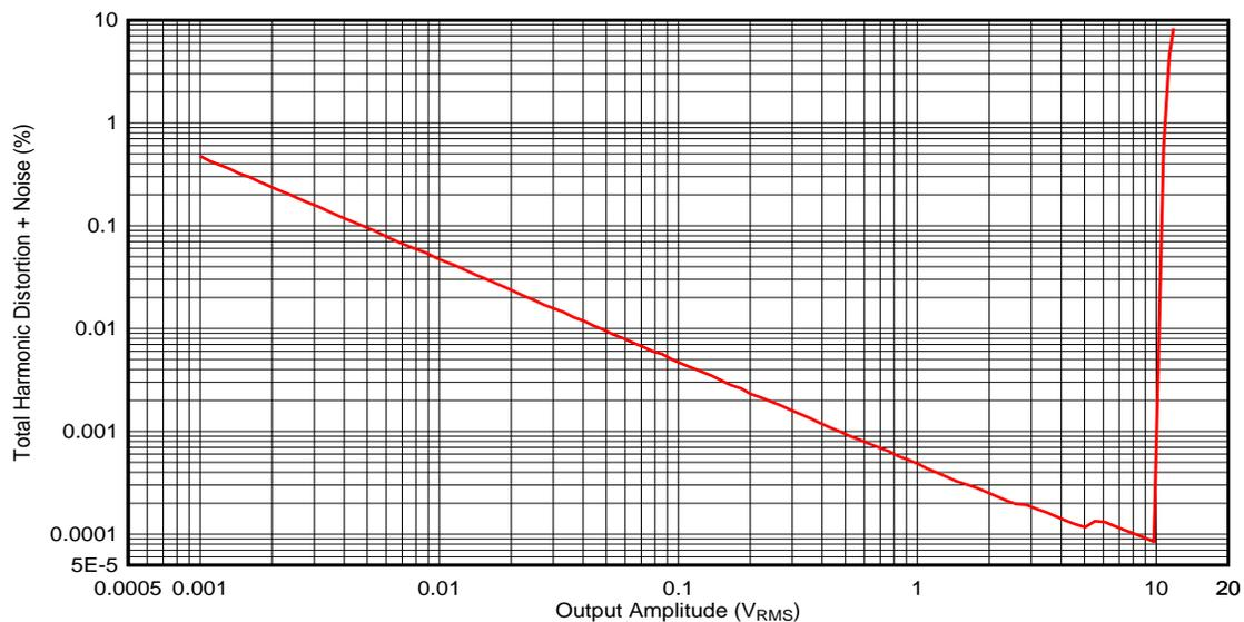
Figure 7. THD+N vs. Amplitude Measurement
