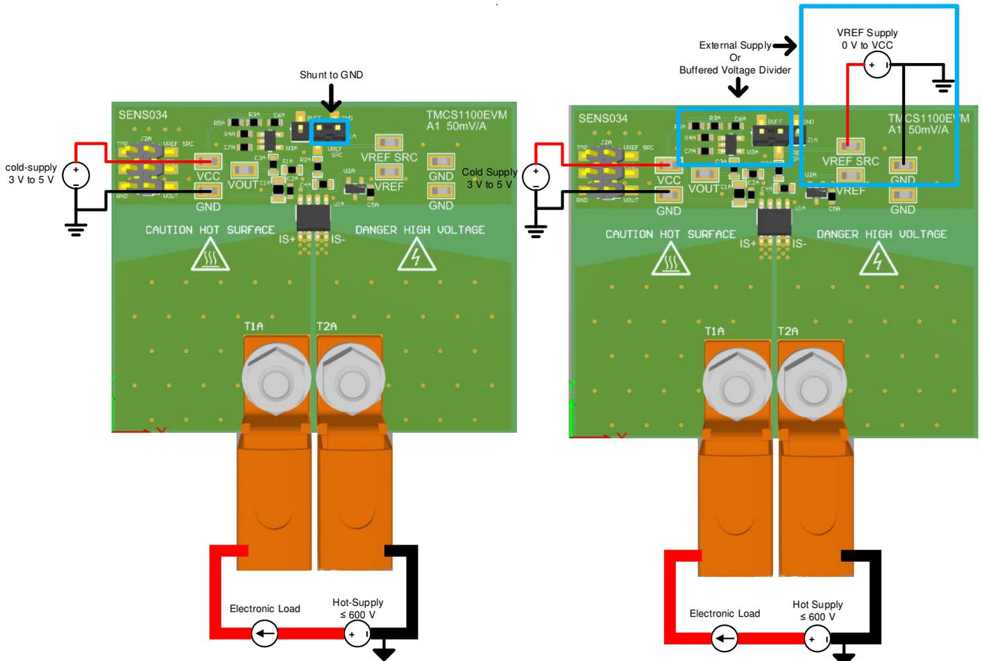
Figure 4-1. Low-Side Unidirectional Setup
