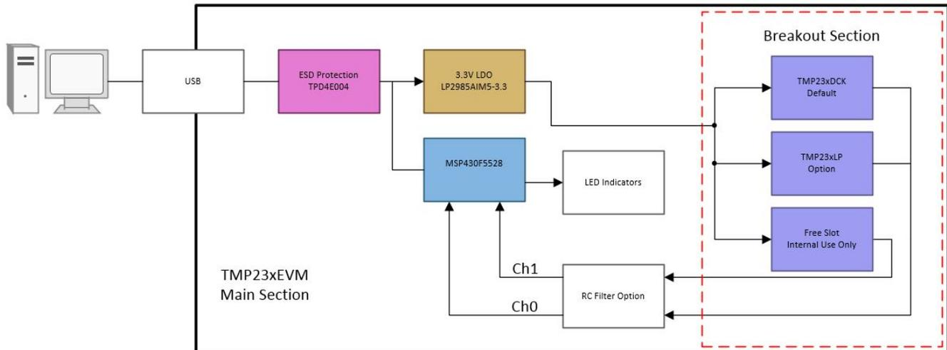
Red dashed lines represent breakable connections on the PCB.
