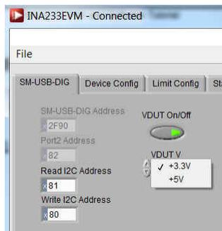
**Figure 4-3. Setting the I<sup>2</sup>C Address**
