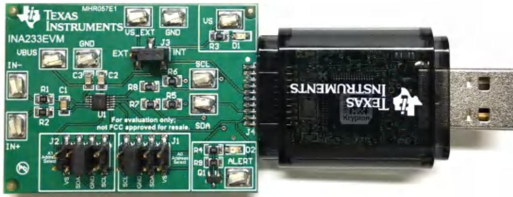
**Figure 3-3. Connecting the INA233 Test Board and SM-USB-DIG Platform Board to the Computer**
