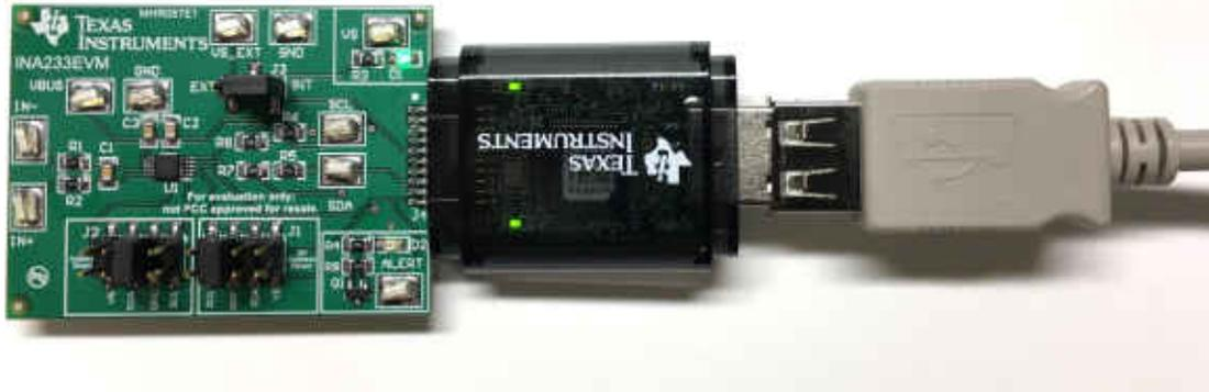
**Figure 3-5. INA233 Power Up Using SM\_USB DIG and INA233EVM GUI Software**
