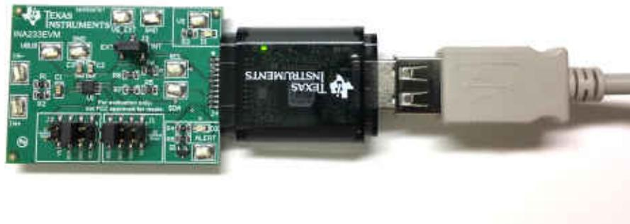
**Figure 3-4. Connecting the INA233 Test Board and SM-USB-DIG Platform Board**
