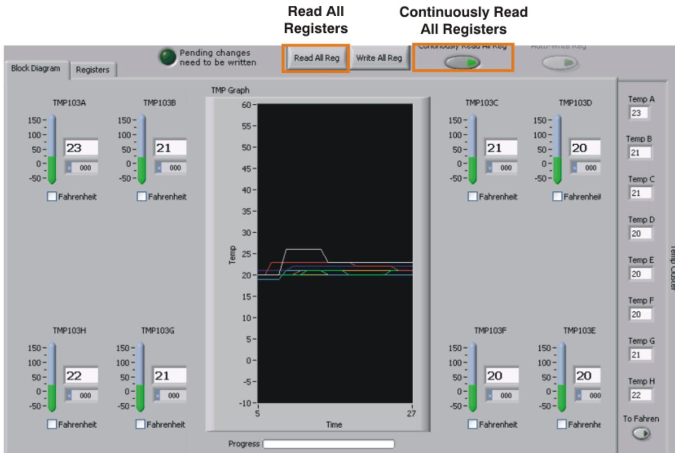
Figure 16. TMP103EVM Software: Reading from Registers
