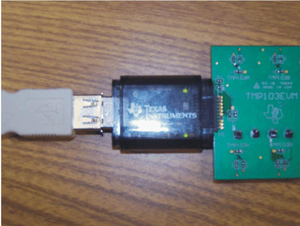
**Figure 5. Connecting the USB Cable to the SM-USB-DIG Platform**
