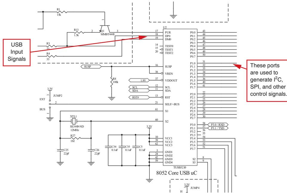
Figure 4. Digital I/O Area—Microcontroller
