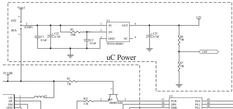
Figure 9. Microcontroller Power
