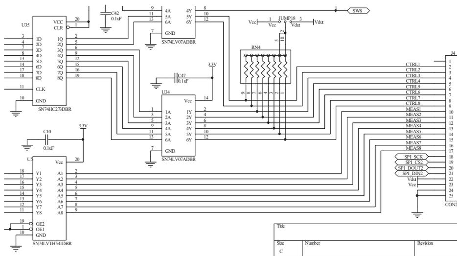
Figure 7. Digital I/O Area—CTRL and MEAS
