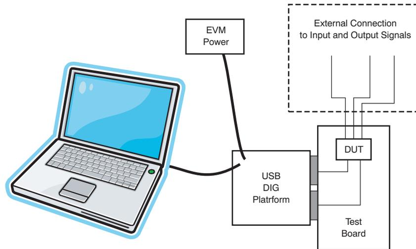
**Figure 2. Hardware Setup for the USB DIG Platform**
