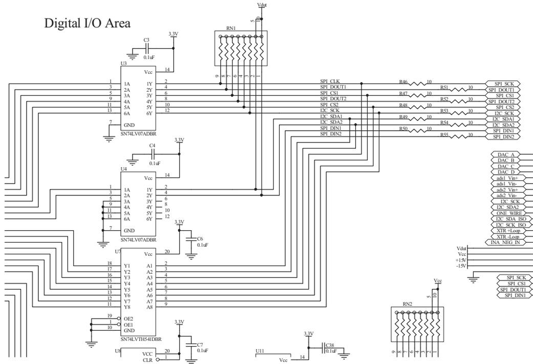
Figure 5. Digital I/O Area—I<sup>2</sup>C and SPI
