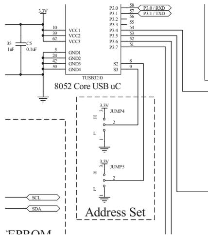
Figure 8. Digital I/O Area—Address Select
