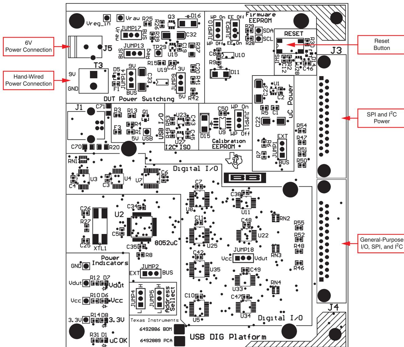
Figure 19. Connector Definition
