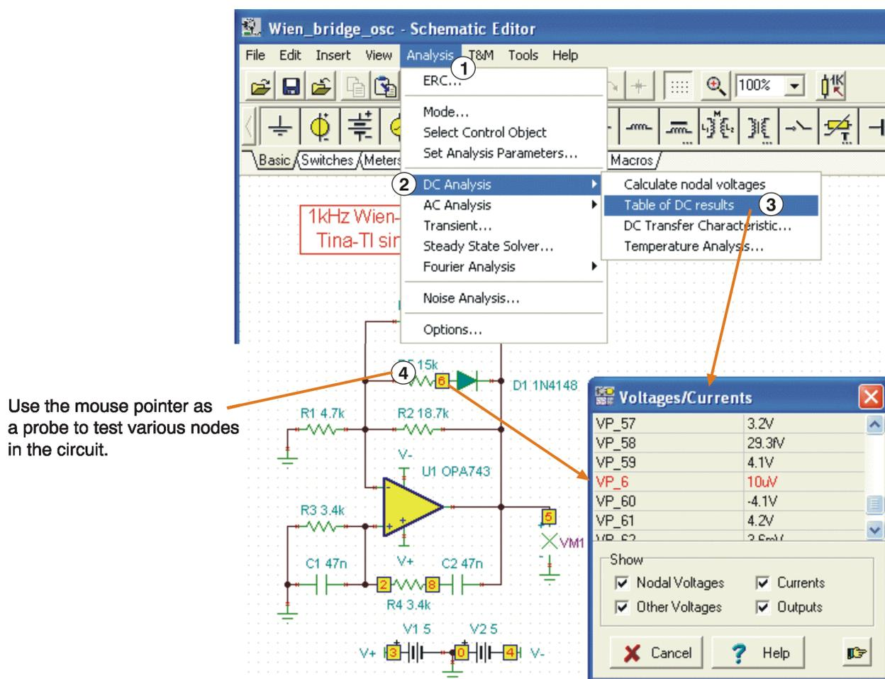
Figure 6. DC Analysis with Voltages/Currents Table Displayed
