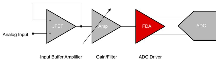
Fully-Differential Amplifier Driving ADC in Example DAQ Front End
