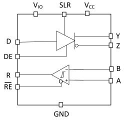
Figure 2-1. Functional Block Diagram of the THVD9491-SEP
