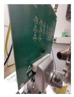
Figure 4-1. THVD9491-SEP Evaluation Board at the TAMU K500 Cyclotron Facility
