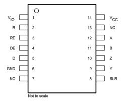
Figure 3-1. THVD9491-SEP Pinout Diagram
