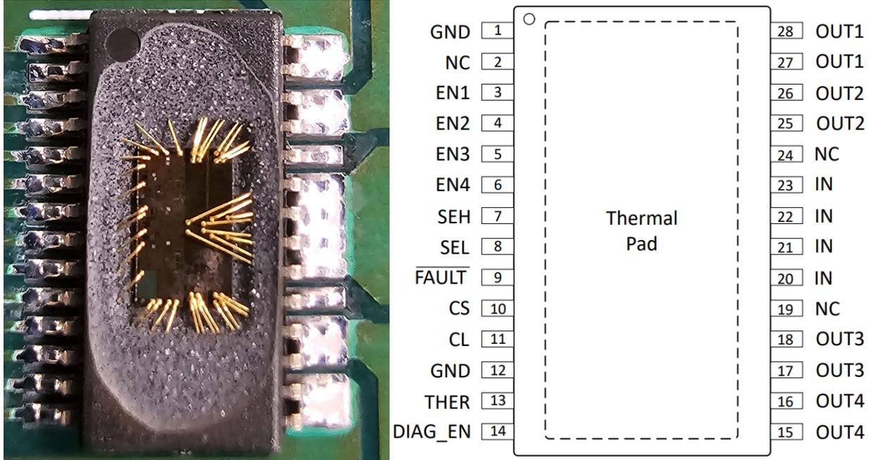
The package was delidded to reveal the die face for all heavy-ion testing.
