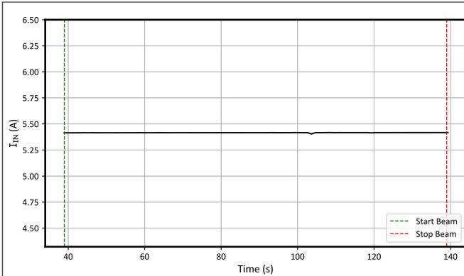
**Figure 7-2.  $I_{IN}$  versus Time for Run 7 (Enabled) for the TPS7H2140-SEP**
