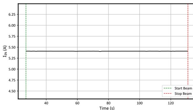
**Figure 7-1. I<sub>IN</sub> versus Time for Run 1 of the TPS7H2140-SEP at T<sub>J</sub> = 125°C**
