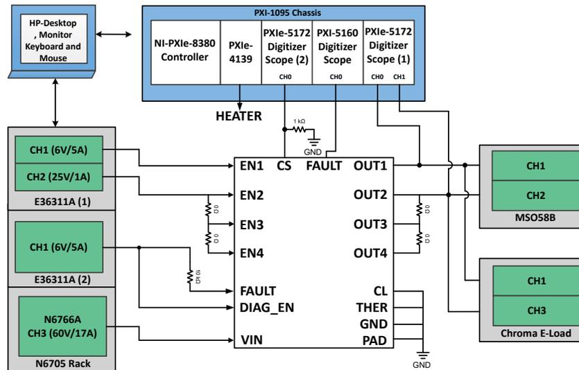
Figure 6-1. Block Diagram of SEE Test Setup with the TPS7H2140-SEP
