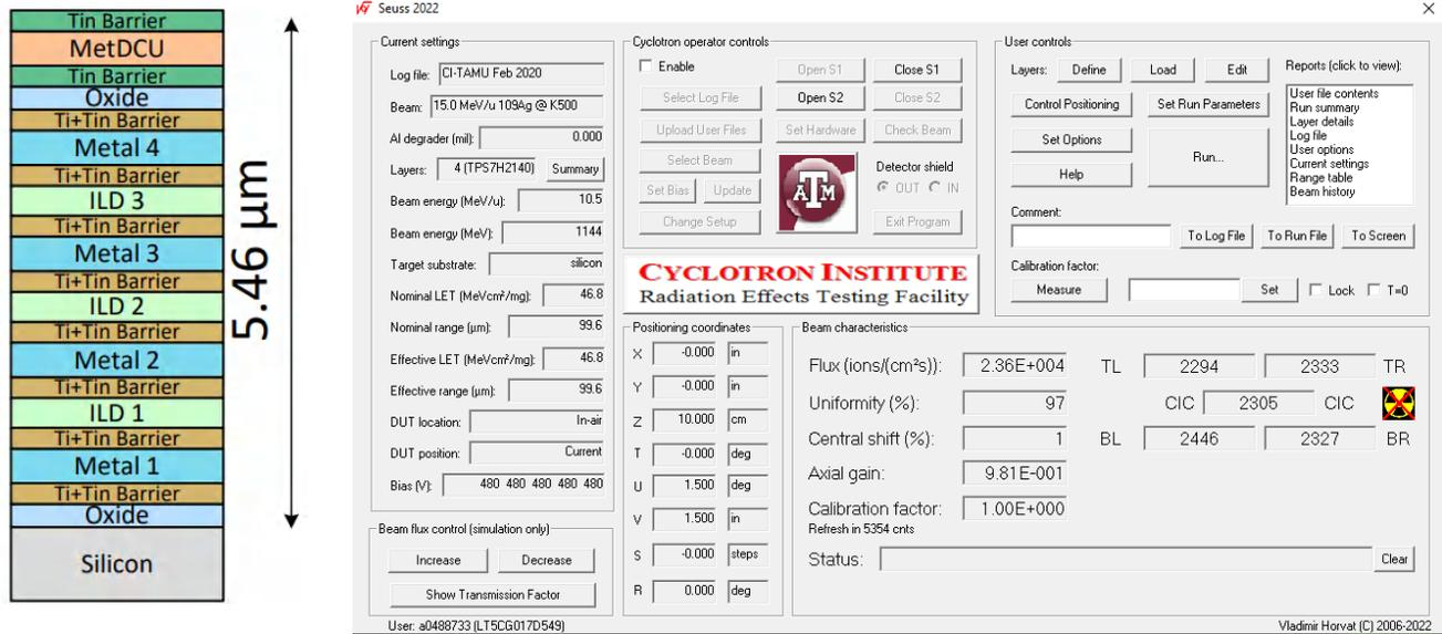
**Figure 5-1. Generalized Cross-Section of the LBC8 Technology BEOL Stack on the TPS7H2140-SEP [Left] and SEUSS 2020 Application Used to Determine Key Ion Parameters [Right]**
