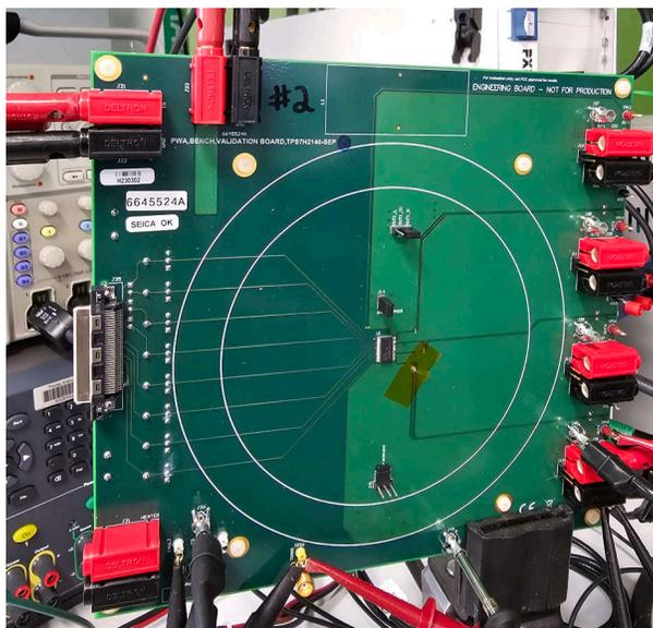
**Figure 4-1. Photograph of the TPS7H2140-SEP Evaluation Board Mounted in Front of the Heavy-Ion Beam Exit Port at the Texas A&M Cyclotron Radiation Effects Facility**
