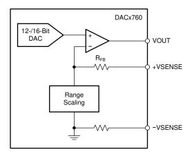
This sense pin is used as a Kelvin connection to provide better accuracy where there are long traces or cables. There are many DACs that are configured with the positive sense pin, but this circuit uses the DAC8760 as an example. The DAC output is set to a range of ±10V.
