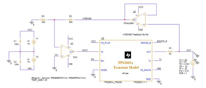
The DAC is set to 0V and a voltage supply is placed at the output of the buffer to simulate an overstress event caused by a wiring error. The supply ramp simulates the overvoltage transition from –32V to +32V.
