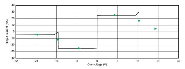
As the voltage increases to near the lower supply voltage of –15V, the TPS26611 begins to conduct current from the DAC output. The DAC, driven by the ramping voltage, immediately reaches the device short-circuit current limit near 30mA. This current limit is lower than the 32mA current limit level of the TPS26611, which passes the conducted current. Sustained operation of the DAC8760 current limit is not destructive.
