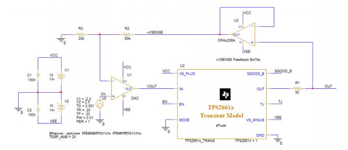
The op amp and resistor network on the left side of the figure represent the voltage DAC output and feedback. The nodes labeled +VSENSE and VOUT are pins for the DAC8760.
