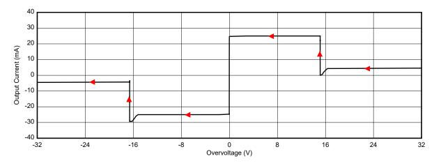
In both simulations, the TVS3301 is not included. The output is not sent beyond the protection threshold of  $\pm 33$ V, which turns on TVS conduction. At the simulated level of 32V, the TVS3301 does not affect the operation of the protection buffer and output of the DAC.
