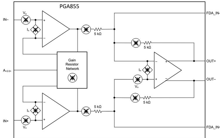
Figure 4-1. Noise Sources for PGA855
