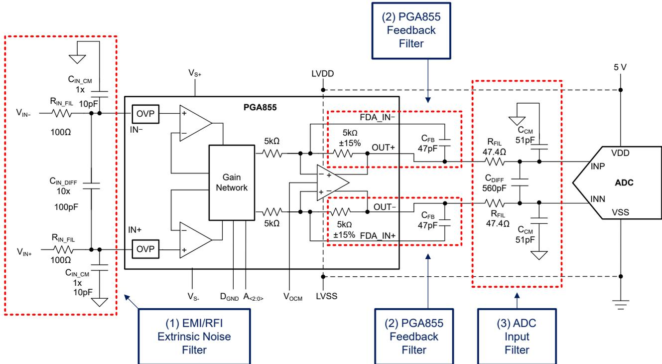
Figure 2-1. PGA855 Analog Filters
