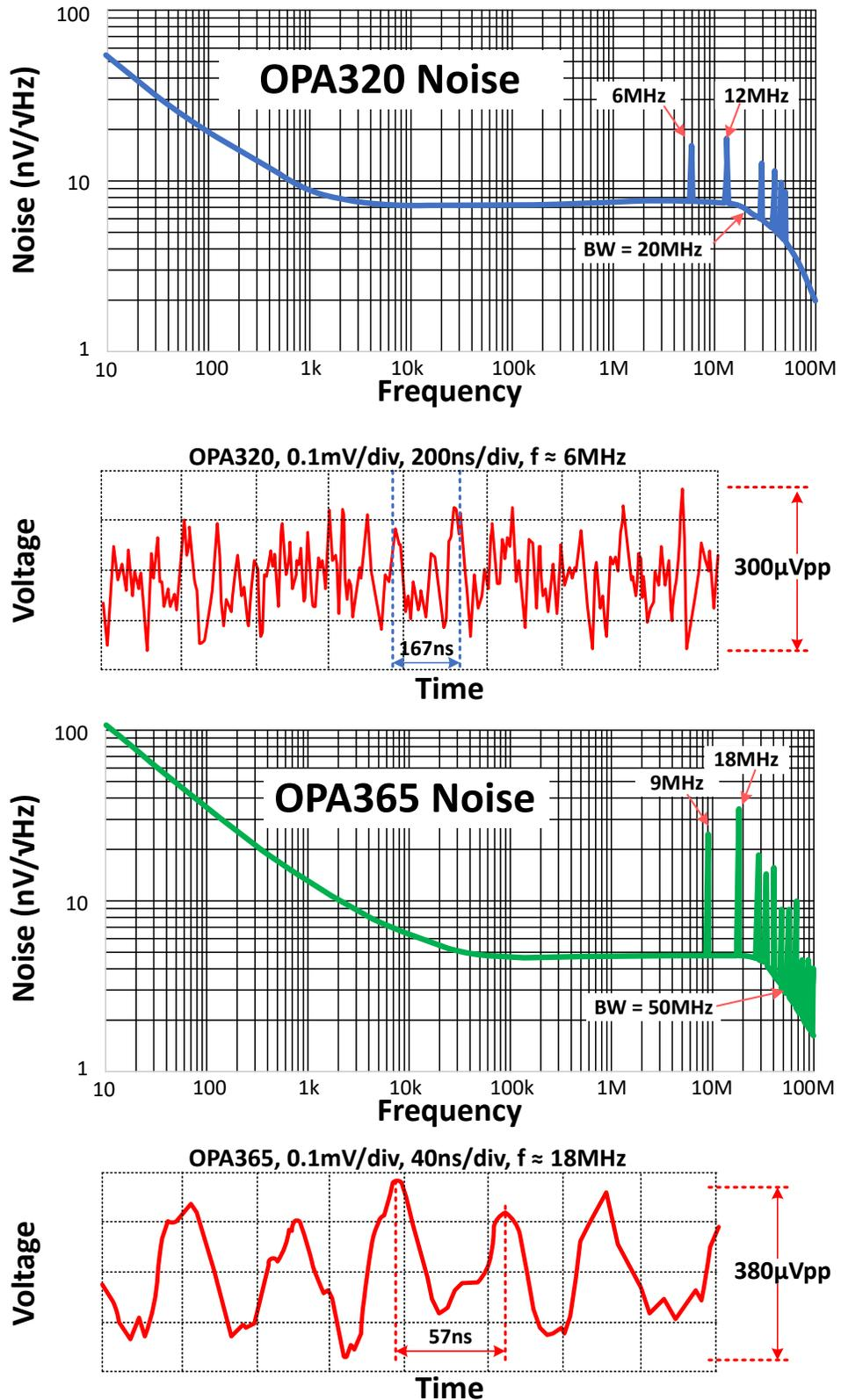
Figure 7-6. Time and Frequency Domain Graph for Device With Internal Charge Pump (Zero-Crossover)
