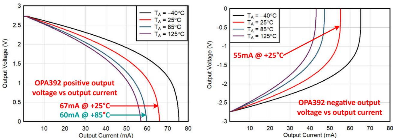
Figure 13-1. Short-Circuit Limit vs Temperature for OPA392
