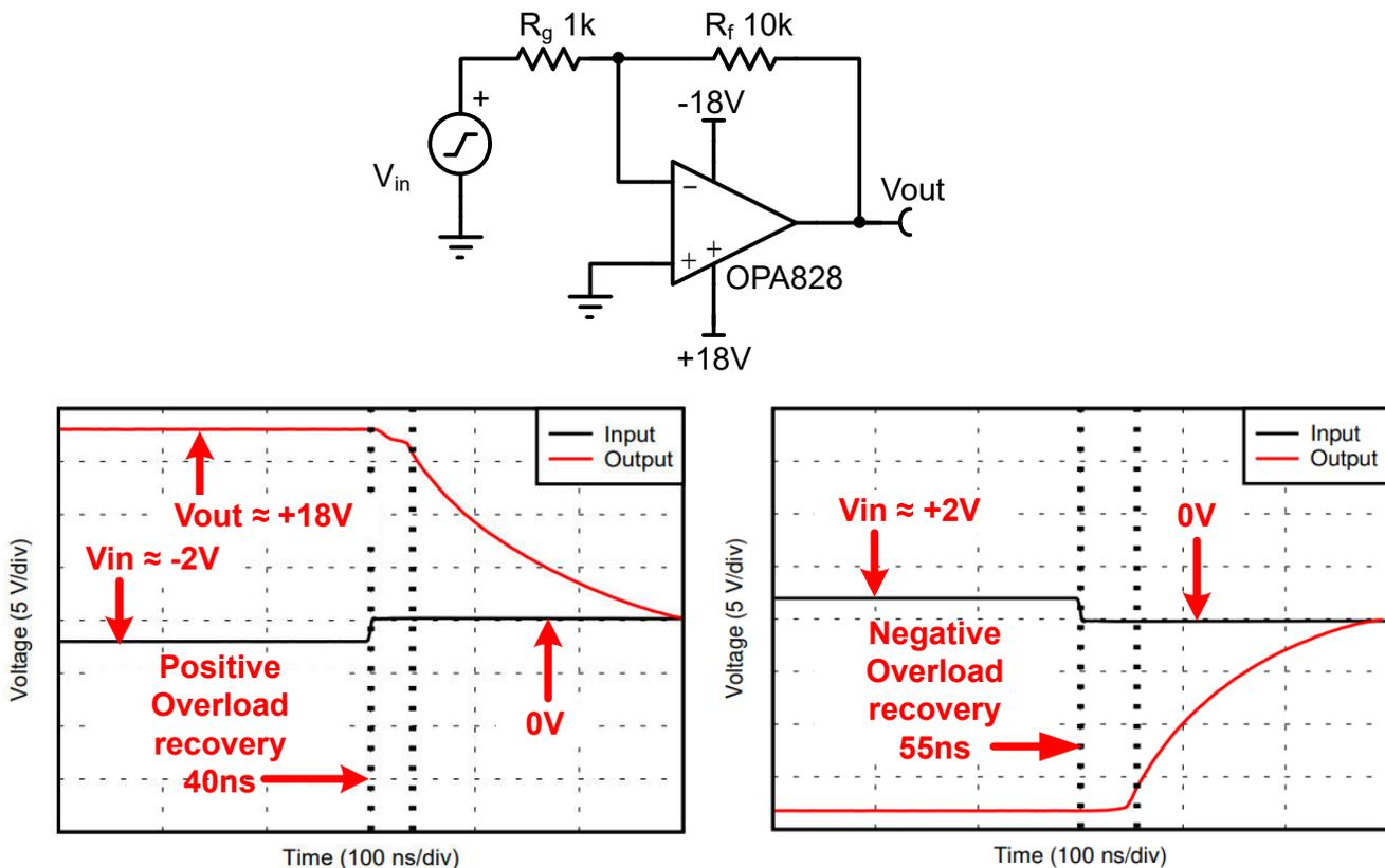
Figure 14-1. Overload Recovery on OPA828
