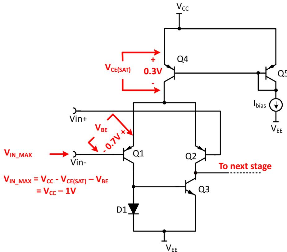
Figure 5-1. Bipolar Input Stage Positive Common-Mode Limit
