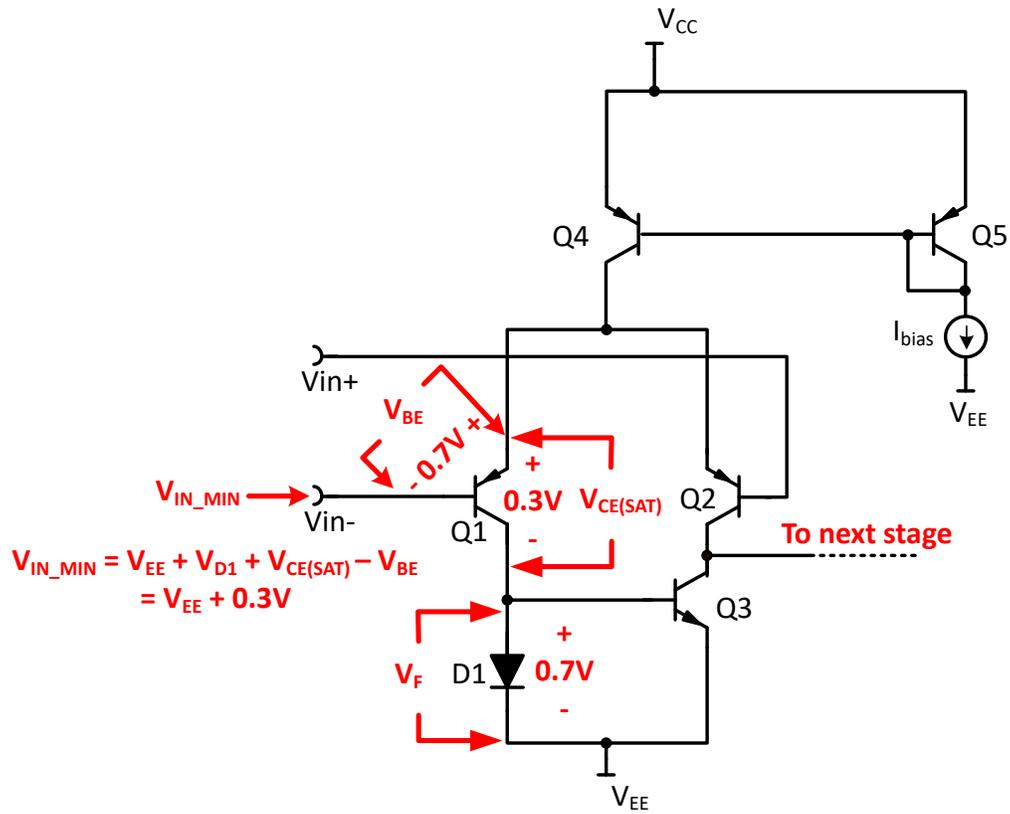
Figure 5-2. Bipolar Input Stage Negative Common-Mode Limit
