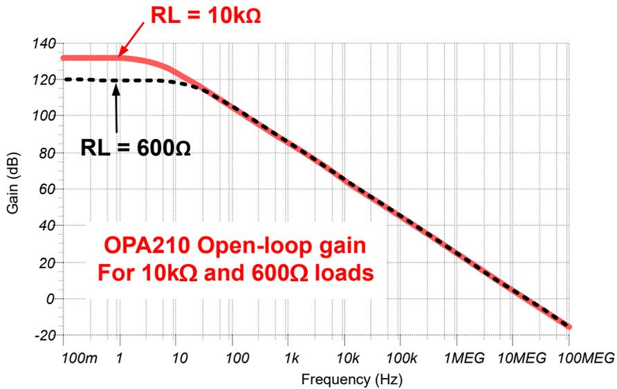
**Figure 12-1. Impact of Loading on  $A_{OL}$  Curve vs Frequency (OPA210)**
