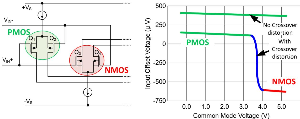
**Figure 7-1. Rail-to-Rail Input Stage With Two Input Pairs and Associated Offset vs Common-Mode Graph**
