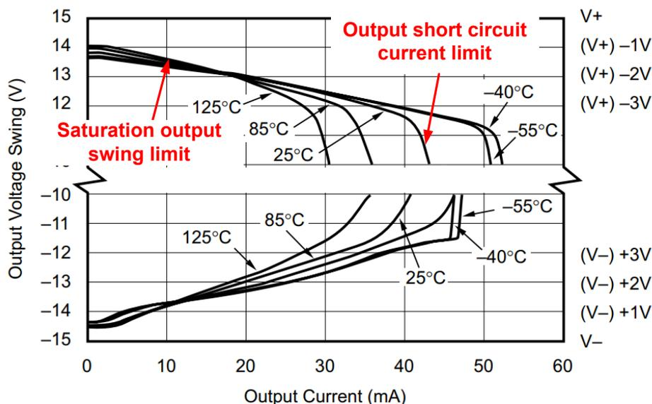
Figure 10-1. Output Voltage Swing vs Output Current for Classic Bipolar Output Stage OPA277
