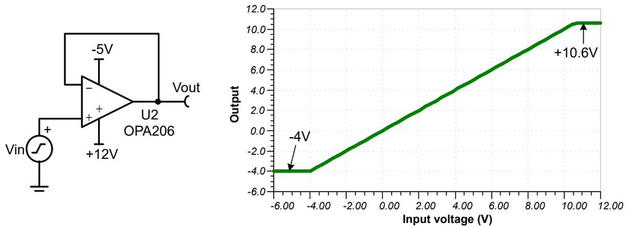
**Figure 2-1. Common-Mode Limit of OPA206 in Buffer Configuration**
