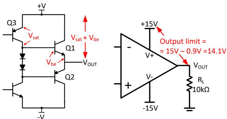
**Figure 8-1. Bipolar Output Stage Example Where Swing is Limited to 0.9 V From Supply**
