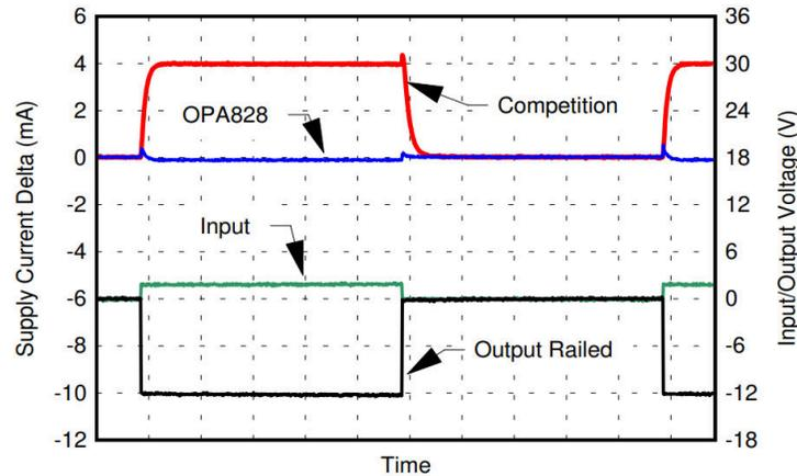
Figure 15-1. Supply Current Change With Overloaded Output (OPA828 vs Competition)
