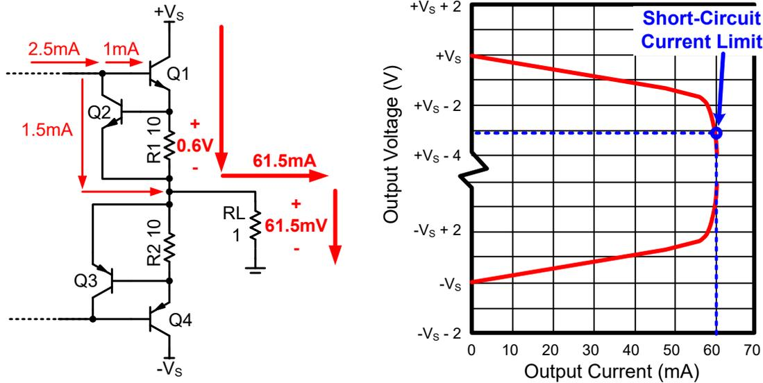
Figure 13-2. Short-Circuit Protection Inside Bipolar Amplifier
