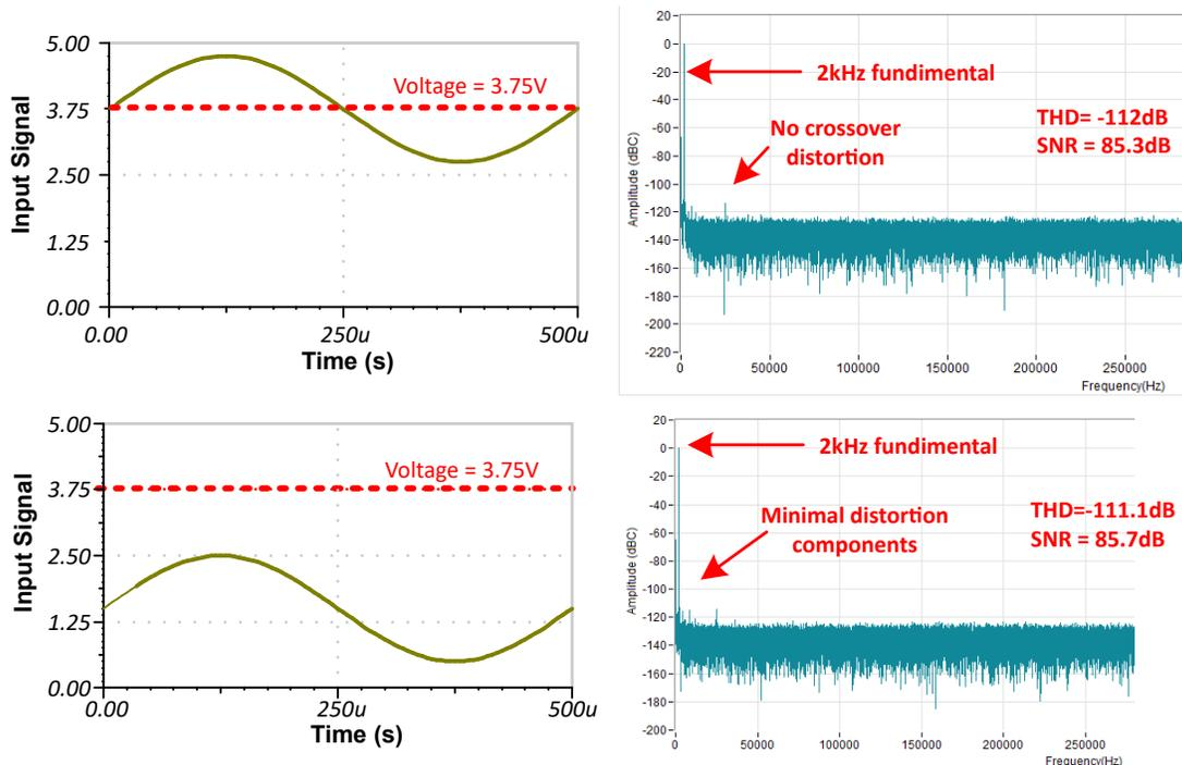
**Figure 7-4. FFT of Signal Inside Applied to a Zero-Crossover Distortion Device (OPA320)**
