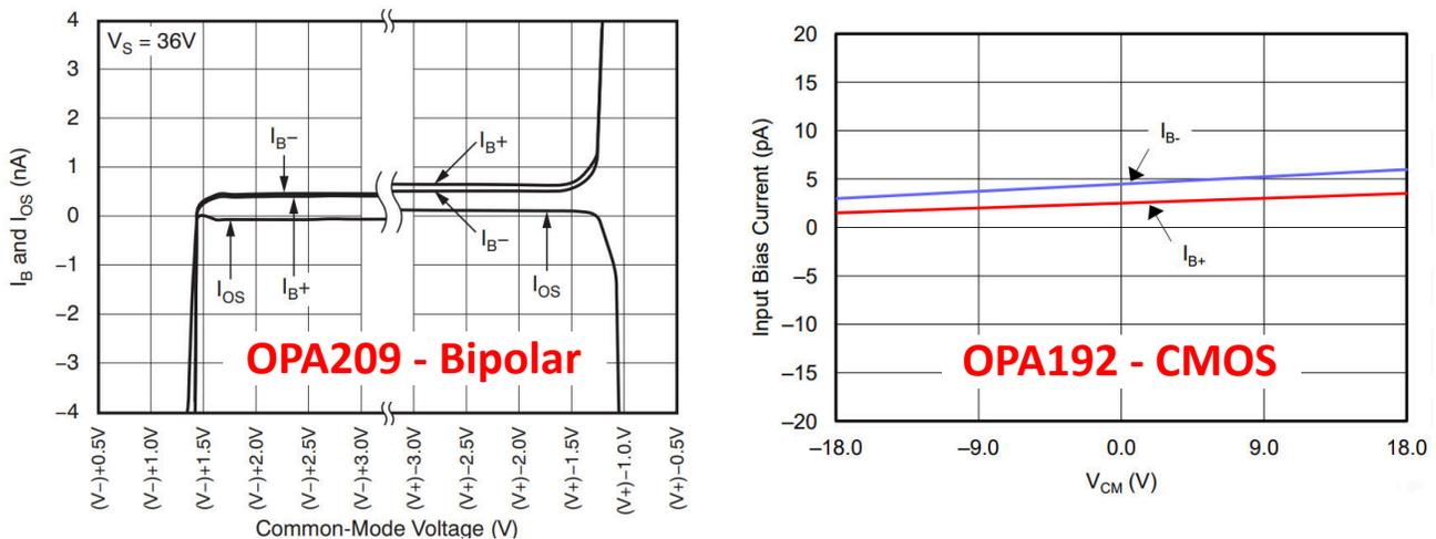
Figure 15-2. Bias Current vs Common-Mode Voltage
