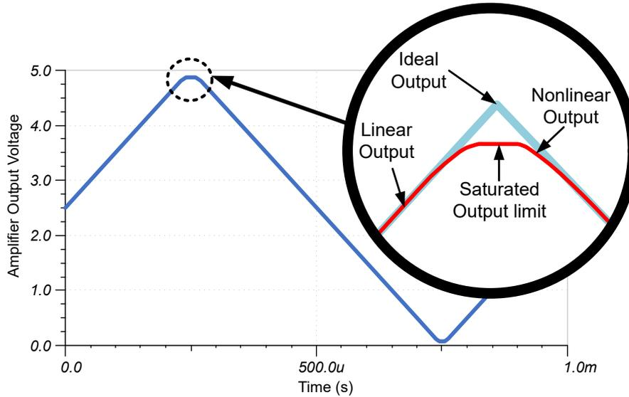
**Figure 9-1. Linear Output Range versus the Saturation Output Swing Limit**
