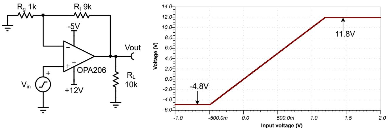
**Figure 2-2. Common Mode Does not Limit OPA206 in Non-inverting Gain of  $10\text{ V/V}$**
