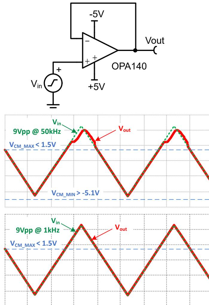
Figure 3-1. Measured Common-Mode Limitation on OPA140 versus Frequency
