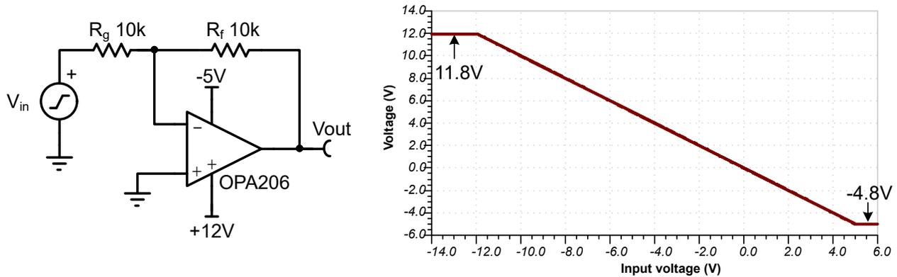
**Figure 2-3. Common Mode Does not Limit OPA206 in Inverting Gain Configuration**
