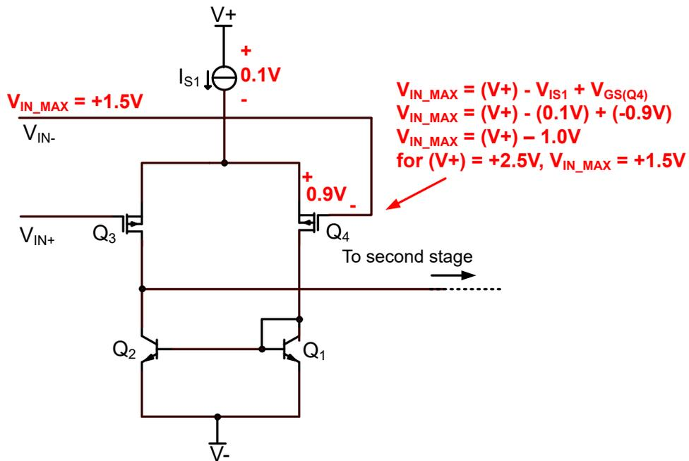
Figure 6-3. Swing to Positive Supply Rail Limitation for P-channel MOSFET
