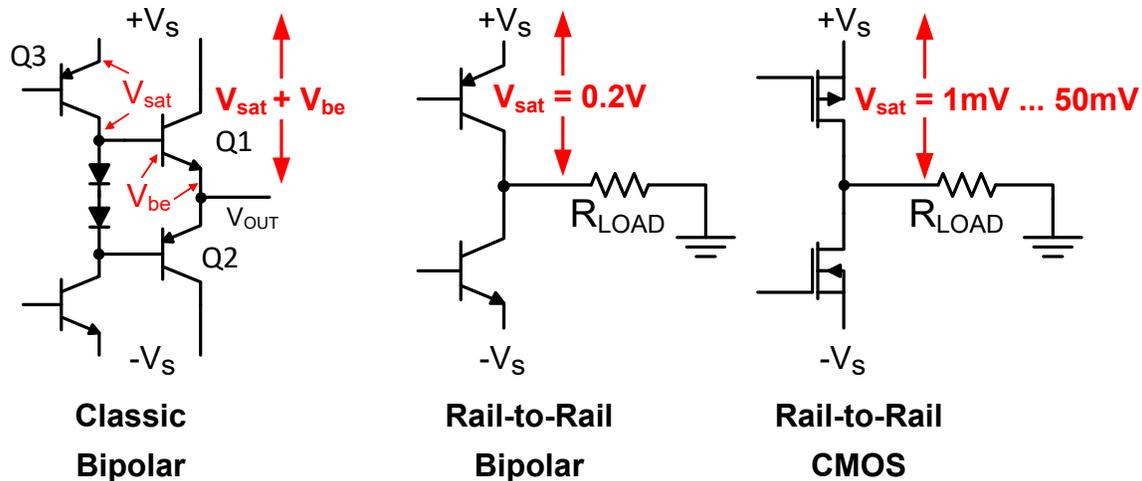
Figure 11-1. Classic Bipolar Output Stage vs CMOS and Bipolar Rail-to-Rail Output Stage
