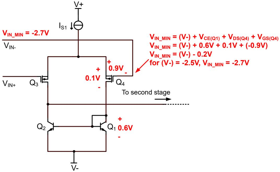
Figure 6-2. Swing to Negative Supply Rail Limitation for P-channel MOSFET
