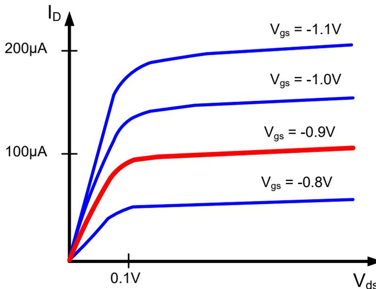
**Figure 6-1. Characteristic Curve for P-channel MOSFET**
