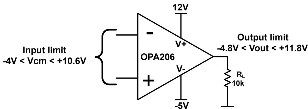
**Figure 1-1. OPA206 Example Common Mode and Output Swing Limits**
