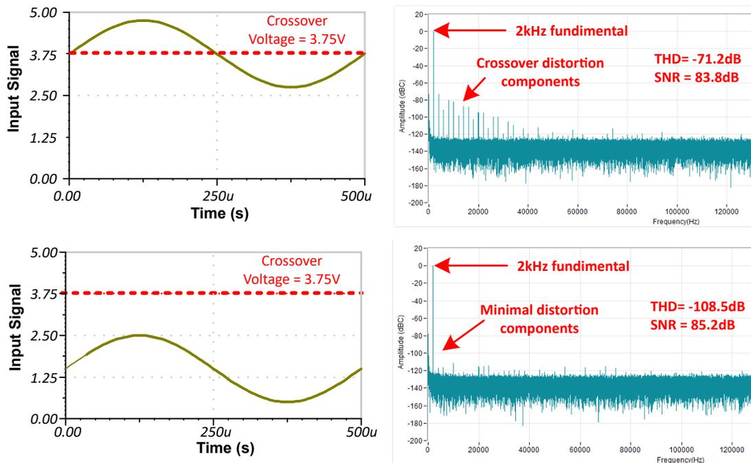
Figure 7-3. FFT of Signal Inside and Outside of the Crossover Region (OPA316)
