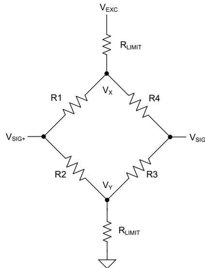
**Figure 2-3. Current Limited Wheatstone Bridge Configuration**
