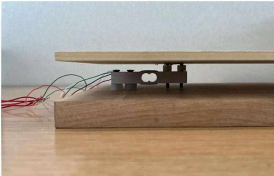
**Figure 8-2. Mechanical Setup for Load Cell**
