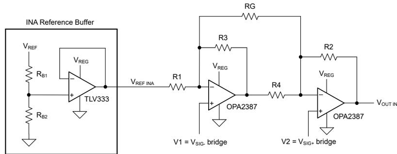
**Figure 2-4. Discrete 2-Amp INA Configuration**
