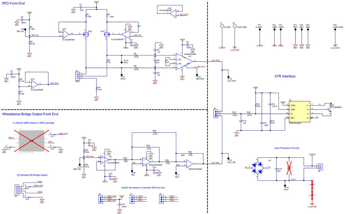
Figure 8-7. PCB Altium Schematic
