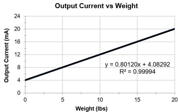
**Figure 5-1. Measured Output Current vs Weight Transfer Function**
