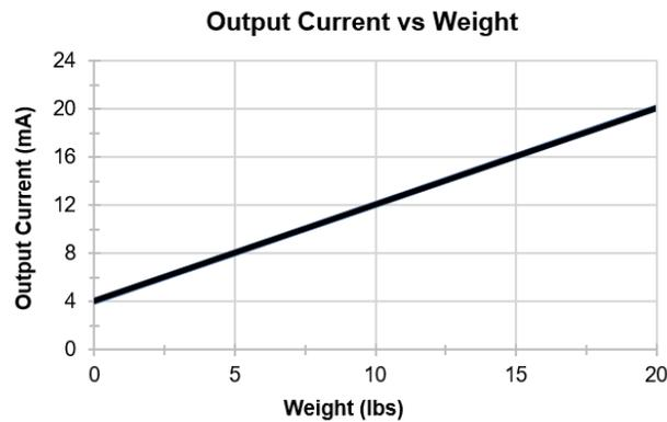
**Figure 1-1. Measured Output Current vs Weight Transfer Function**
