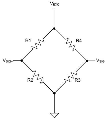
**Figure 2-2. Basic Wheatstone Bridge Configuration**
