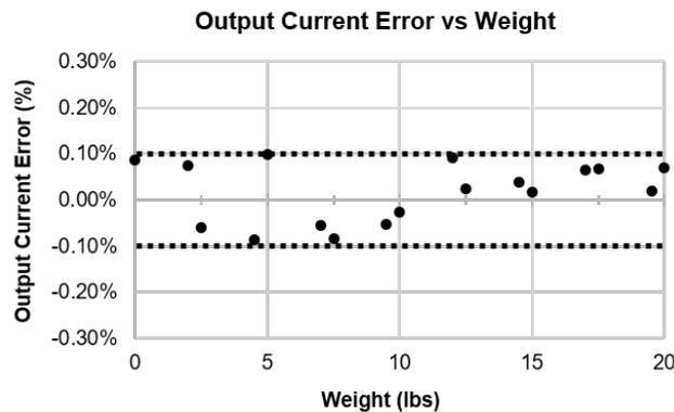
**Figure 5-2. Output Current Error vs Weight**
