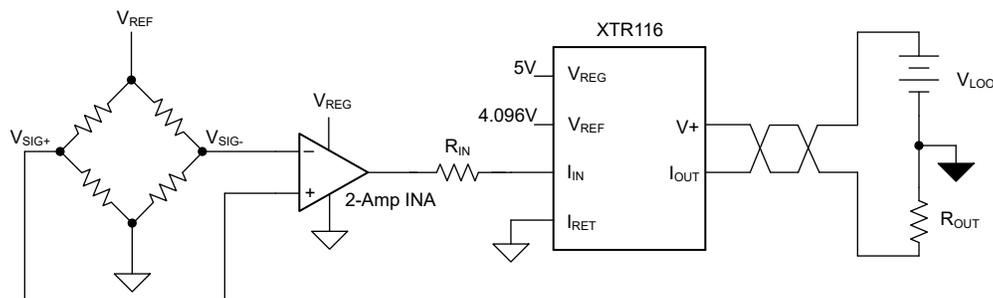
Figure 2-1. Simplified Bridge Amplification to 4-20-mA Circuit
