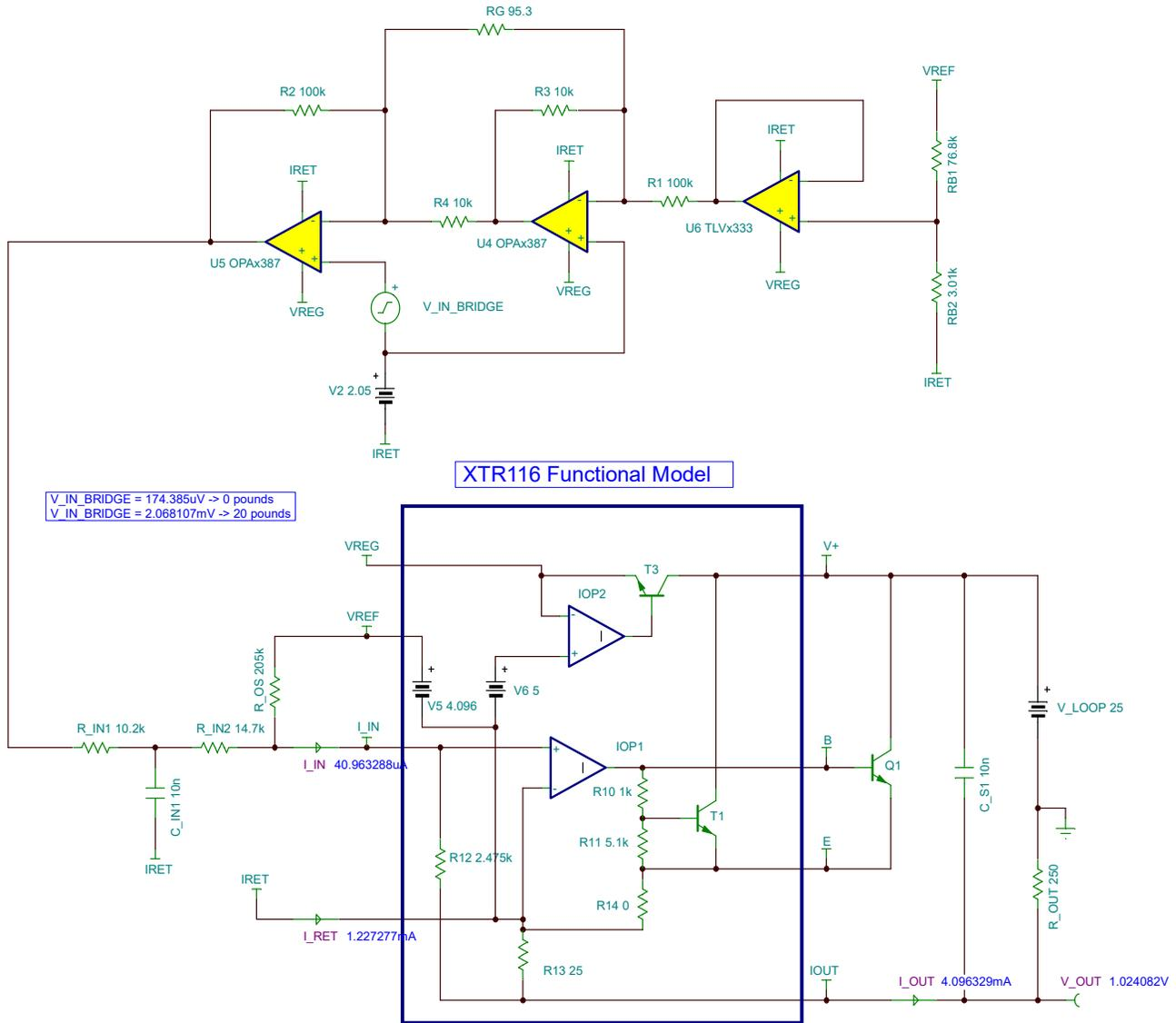
Figure 3-1. TINA TI Schematic and Simulation for 0-lbs Input
