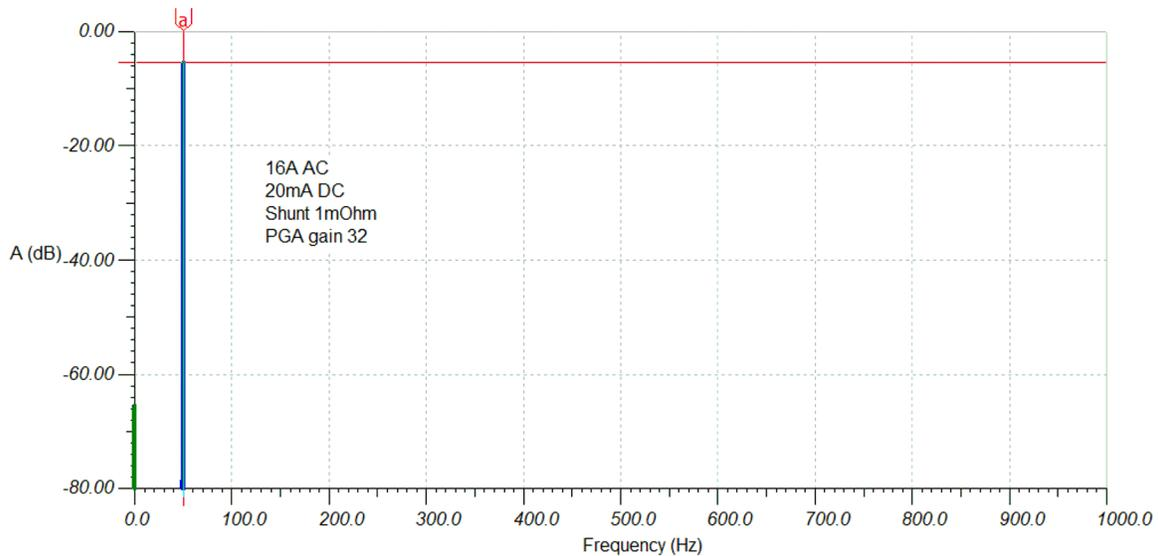
**Figure 3-1. FFT DC in AC with PGA Gain = 32, VREF = 1.2 V**
