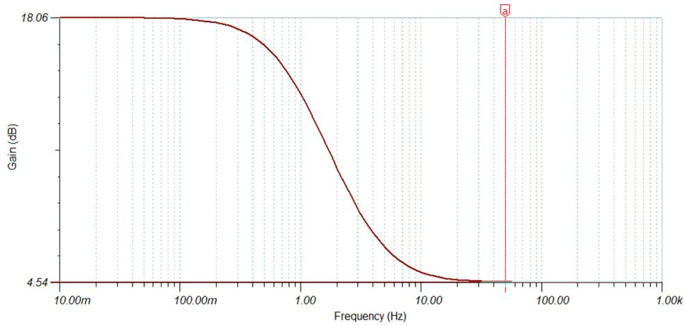
**Figure 3-3. Frequency Response of the First Order Shelving Filter**
