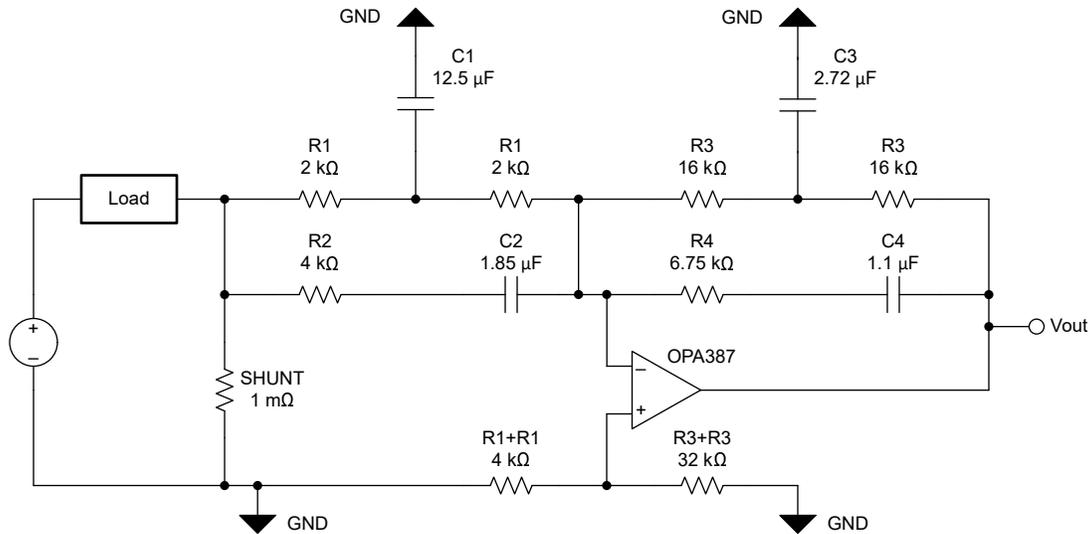
Figure 3-6. Second Order Shelving Filter Circuit
