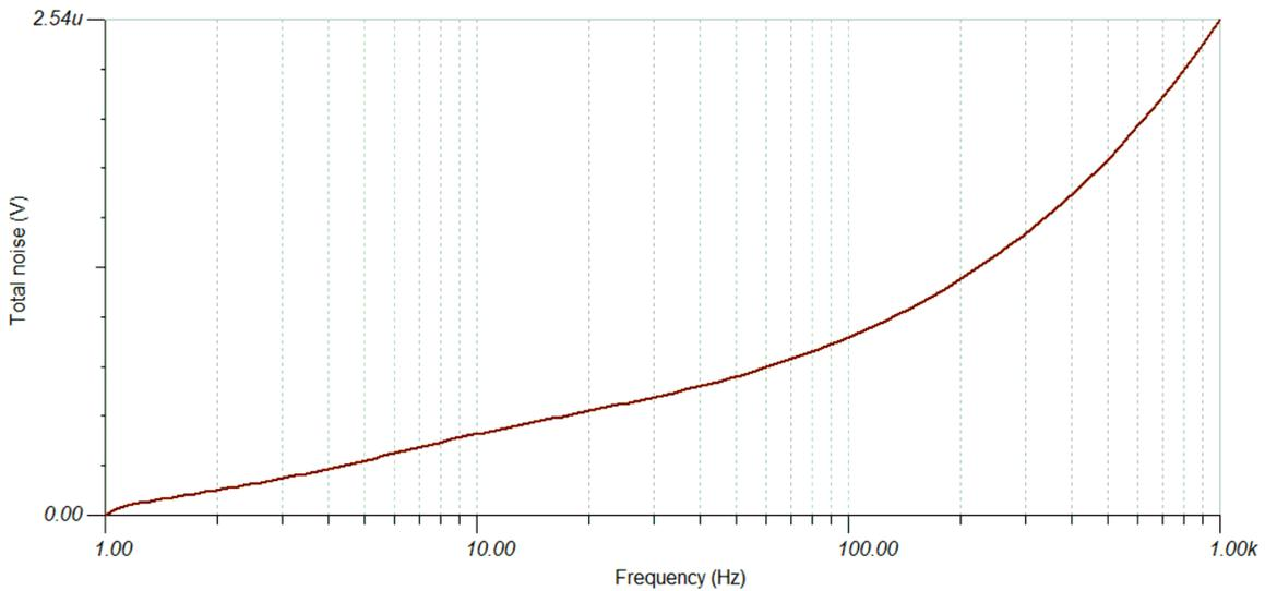
**Figure 3-9. Total Output Noise of the Second Order Shelving Filter**
