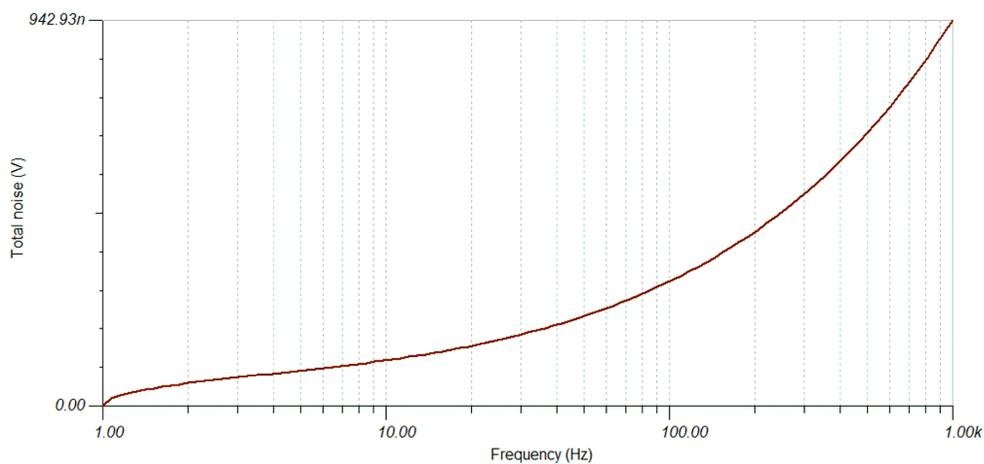
**Figure 3-5. Total Output Noise of the First Order Shelving Filter**
