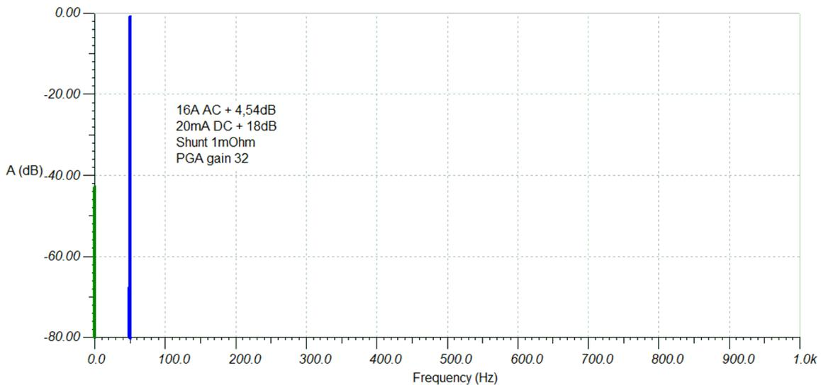
**Figure 3-11. FFT DC in AC With PGA Gain = 32 and Filter Correction, VREF = 1.2 V**
