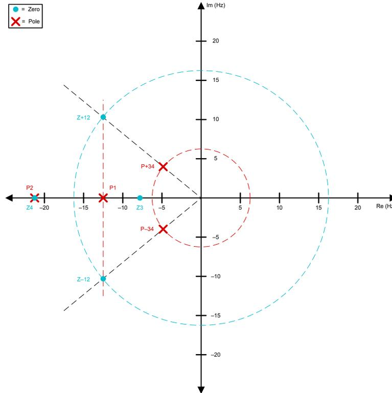
**Figure 4-1. Pole-Zero-Plot of the Second Order Shelving Filter**
