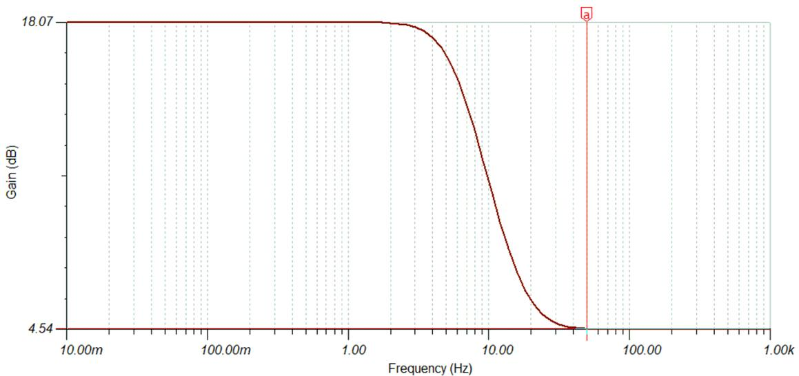
Figure 3-7. Frequency Response of the Second Order Shelving Filter
