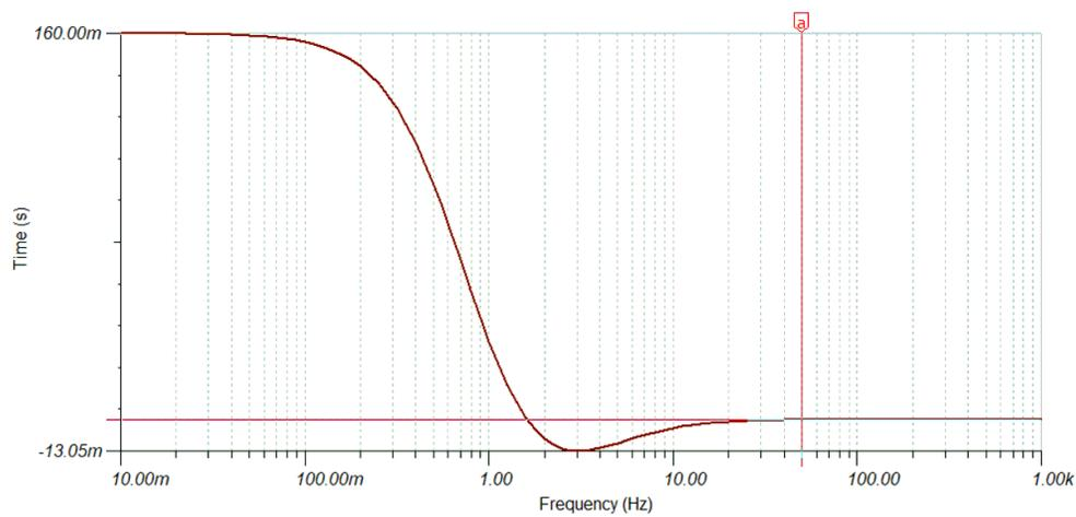
**Figure 3-4. Group Delay of the First Order Shelving Filter**
