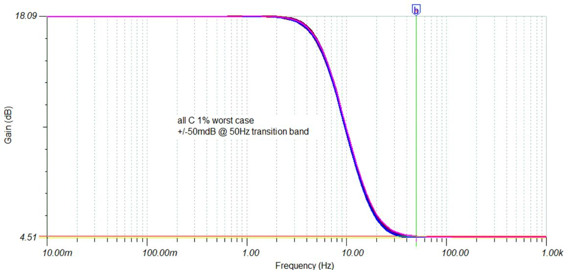
**Figure 5-2. Frequency Response Worst Case Deviation With All C = 1%**
