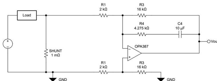
**Figure 3-2. First Order Shelving Filter Circuit**
