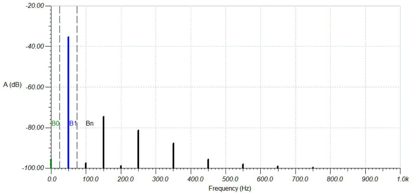
**Figure 2-1. FFT DC in AC + Harmonics, VREF=1.2V**
