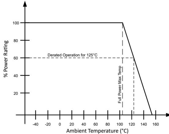
**Typical Shunt Derating Curve**
