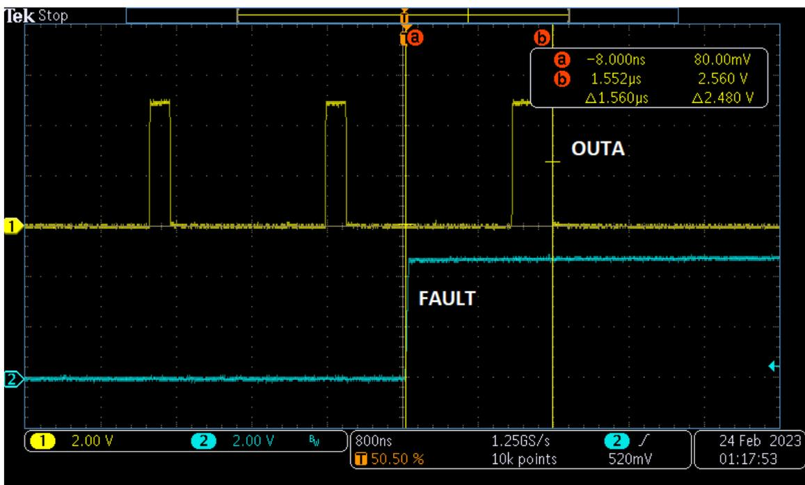
Figure 4. TPS7H500x-SP FAULT Pin Response Time
