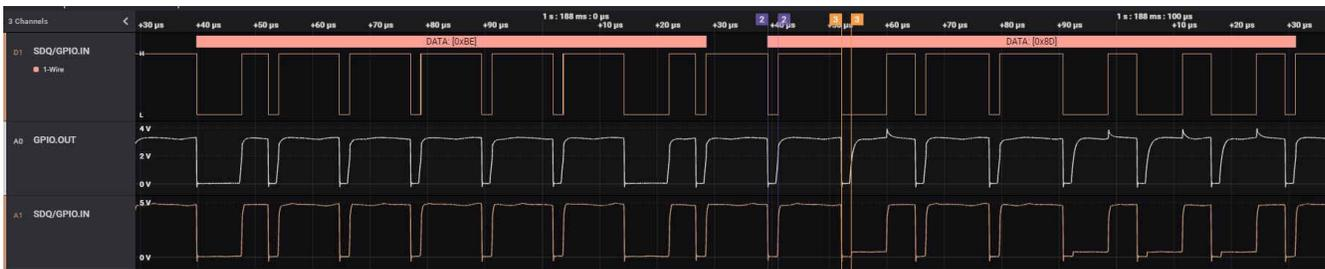
Figure 2-5. Scope Capture of Read Transfer
