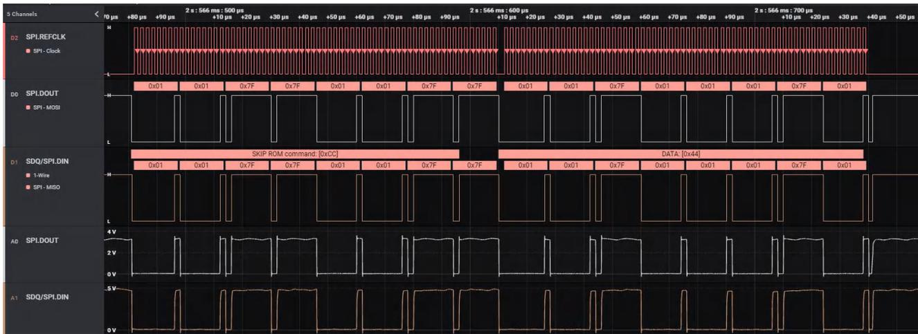
Figure 2-16. Scope Capture of Write Transfer
