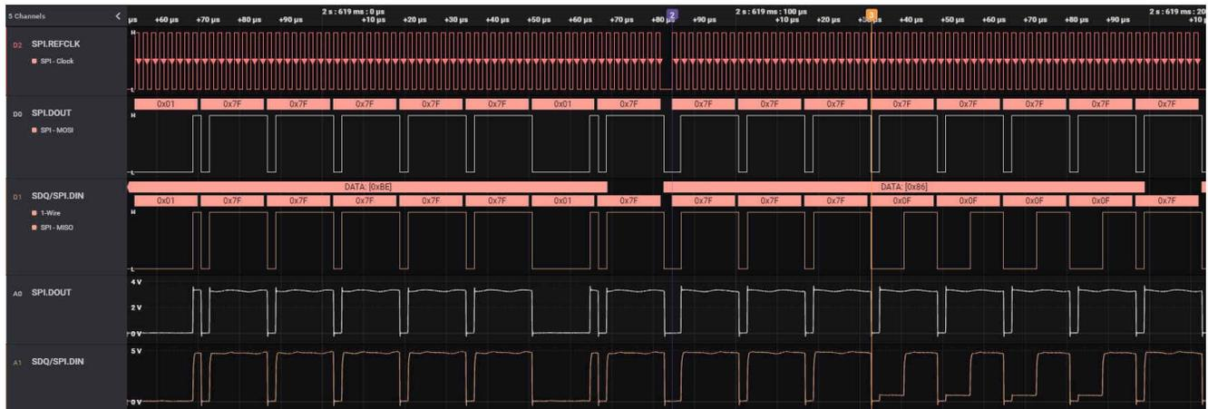
**Figure 2-17. Scope Capture of Read Transfer**
