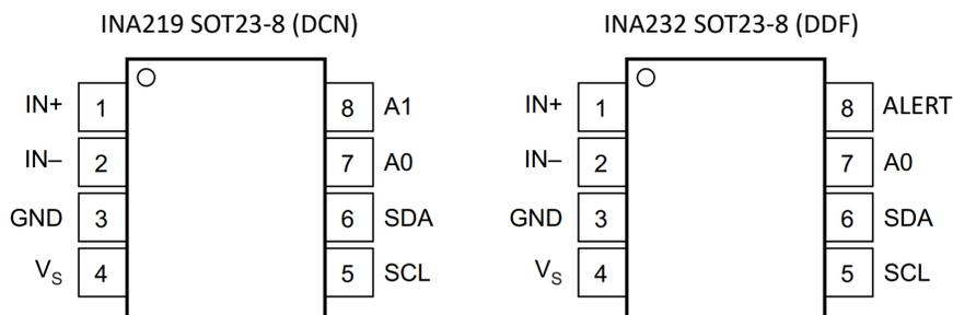
**Figure 2-1. Package and Pinout**
