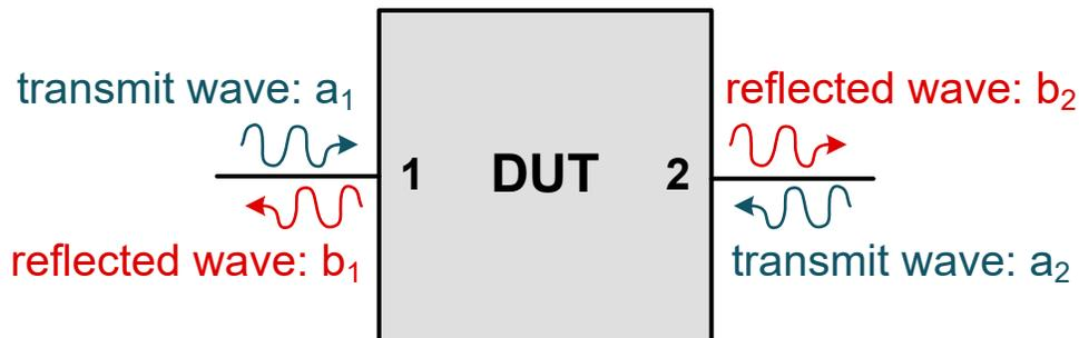
Figure 3. Two-Port Network Wave Quantities
