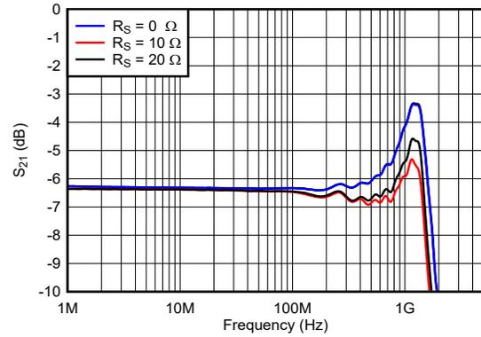
Figure 5. Peaking in  $S_{21}$  due to  $L_S$  and  $C_{IN}$  Resonance
