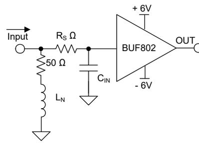
**Figure 10. Effective Input Impedance with  $R_S$  and  $L_N$**
