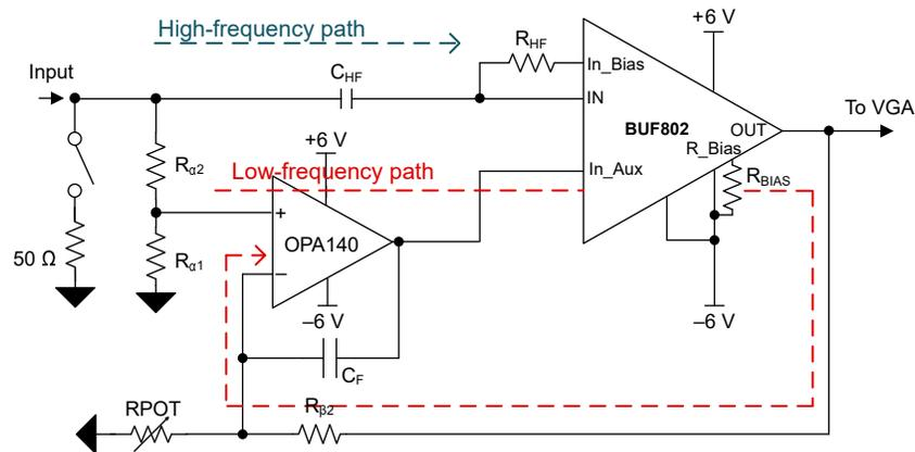
Figure 2. Composite Loop Low- and High-frequency Paths
