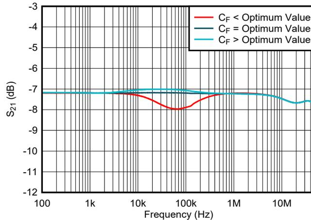
**Figure 8. Tuning Output Response with Different  $C_F$  Value**
