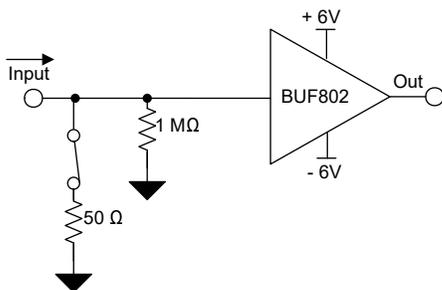
**Figure 9. BUF802 with Optional 1 M $\Omega$  / 50  $\Omega$  Termination**
