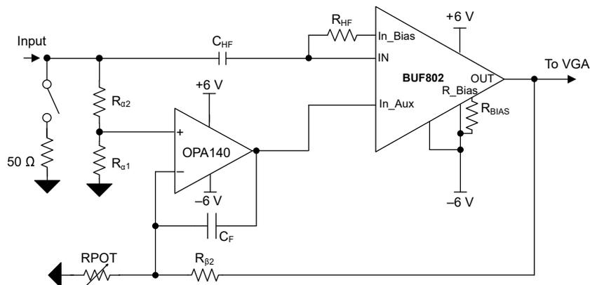
**Figure 1. Generic Composite Loop Front-End Stage with OPA140 and BUF802**
