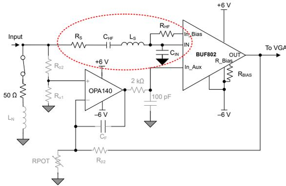
Figure 4. Input Parasitic Network
