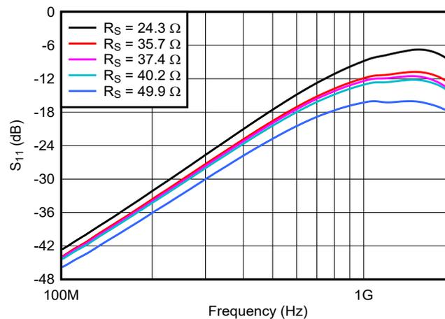
**Figure 11.  $S_{11}$  with Varying  $R_S$**
