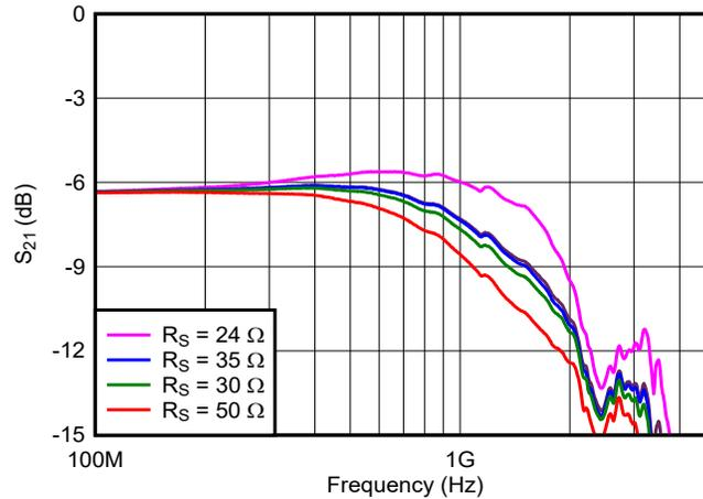
Figure 6.  $S_{21}$  Input Response with Varying  $R_S$
