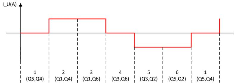
**Figure 7-2. Ideal BLDC Motor Phase Current**
