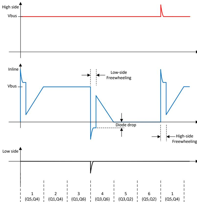
Figure 7-5. Common-Mode Voltage (Not to Scale)
