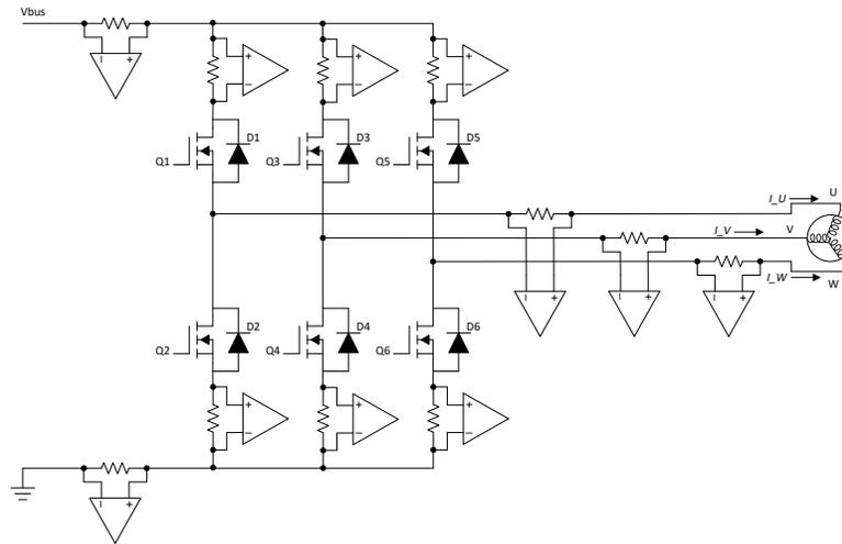
**Figure 7-1. Common Motor Current-Sensing Topologies**
