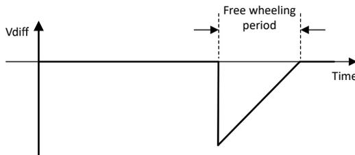
Figure 7-6. Negative Differential Input Voltage due to Decaying Phase Current
