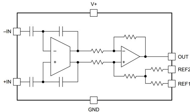
Figure 4-3. Switched Capacitor CSA
