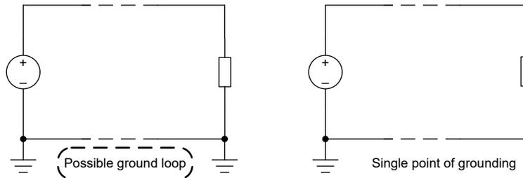
**Figure 2-2. Ground Loop and its Prevention**
