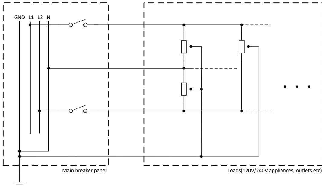
**Figure 1-1. One-Line Diagram Of Utility Household Electric System in the US**
