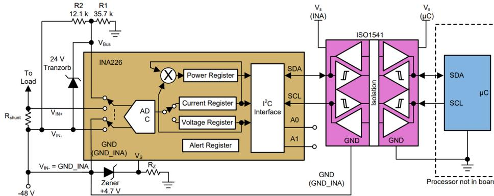
Figure 6-1. -48-V Power-Sensing Reference Design
