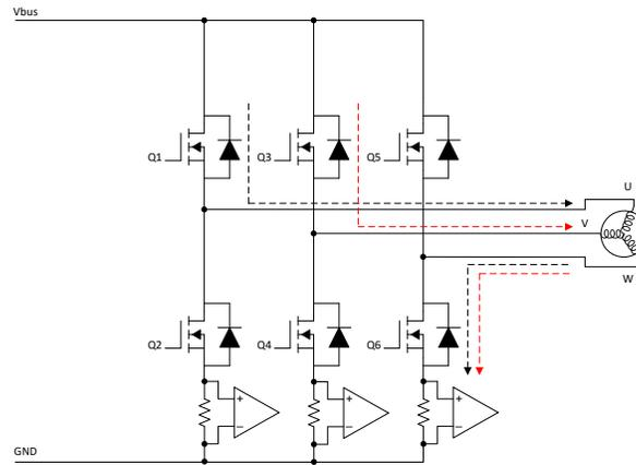
**Figure 7-3. Switching of Motor Phase Currents**
