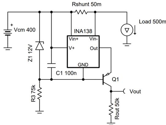
**Figure 6-2. 400-V Current Sensing**
