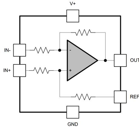
**Figure 4-1. Single-Stage Diff Amp Based CSA**
