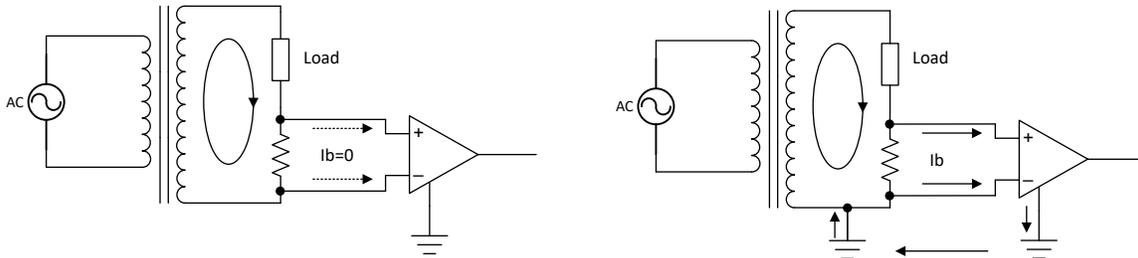
**Figure 5-1. Without (Left) and With (Right) Return Path for Input Bias Current**
