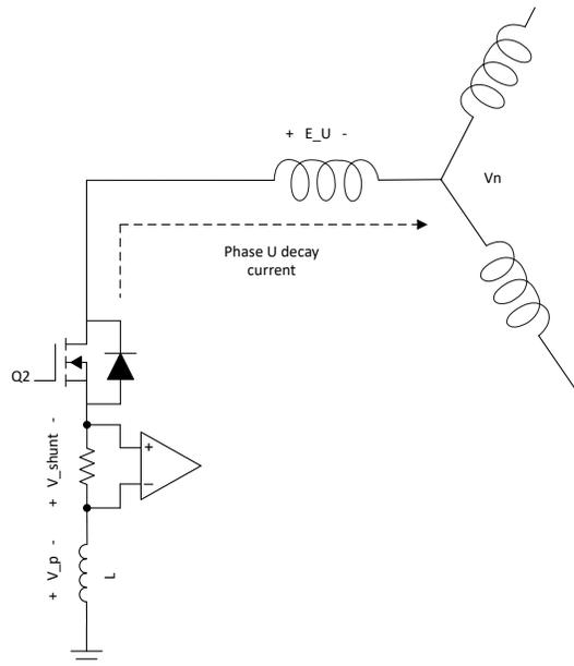
**Figure 7-4. Freewheeling Current Through Low-Side Diode**
