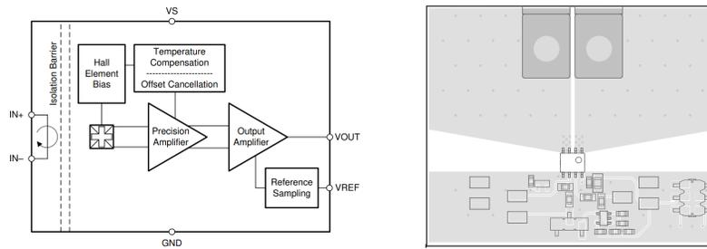
**Figure 3-2. Hall-Effect Current Sensor TMCS1100 Block Diagram and PCB Layout**
