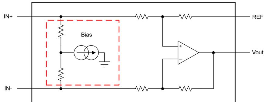
Figure 4-4. Bias and Common-Mode Sensing in CSA
