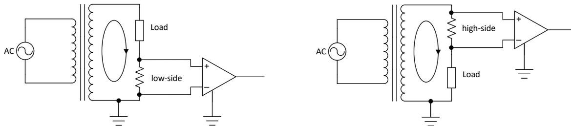
**Figure 5-4. Grounded Secondary Coil for Low-Side (Left) or High-Side (Right) Current Sensing**
