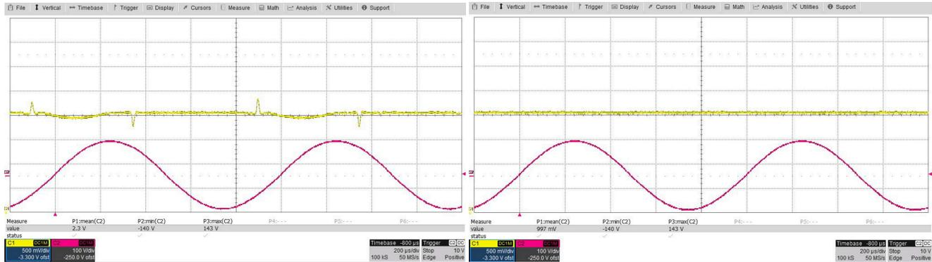
**Figure 5-3. Output Waveform With Floating (Left) and Grounded (Right) Input**
