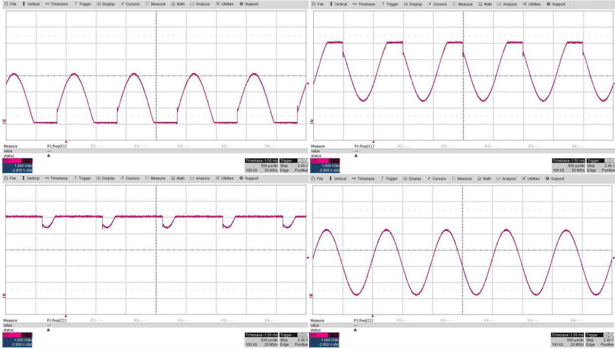
Figure 5-6. Unpredictable Output of AC-Coupled CSA
