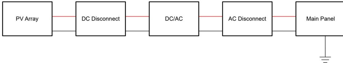
**Figure 2-1. A Grounding Scheme of Grid-Tied PV System**
