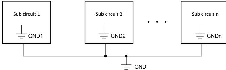
**Figure 2-4. PCB STAR Grounding**
