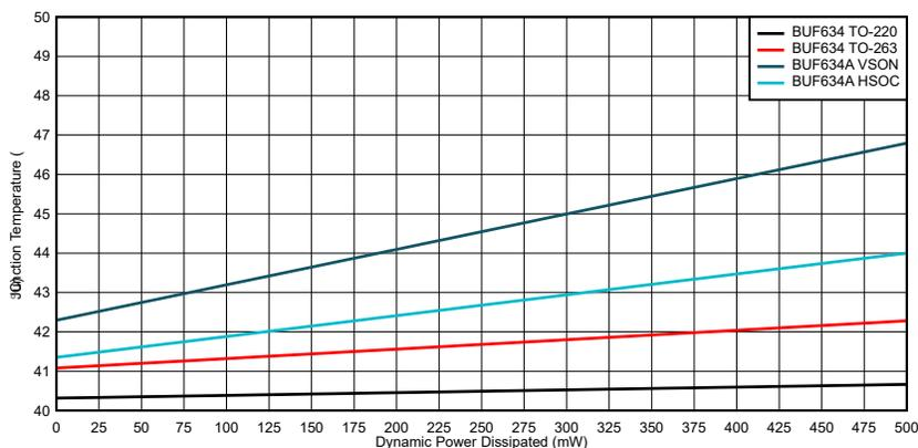
**Figure 2-1. TO-220, TO-263, VSON, HSOIC0 Junction Temperature Comparison for 40 °C Board Temperature**
