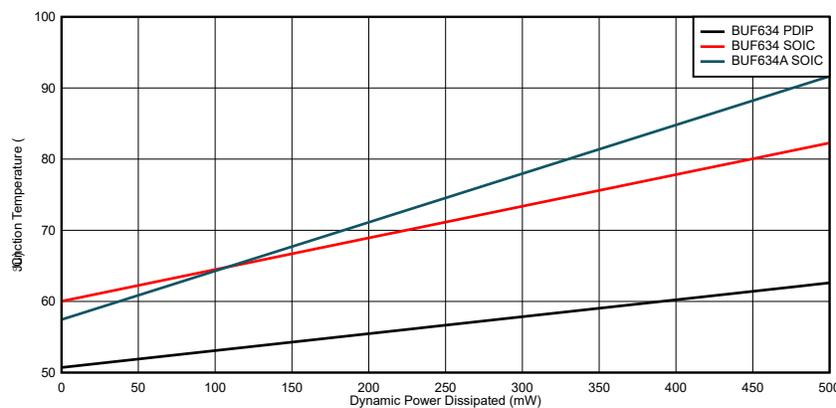
**Figure 2-2. BUF634 PDIP, SOIC and BUF634A SOIC Thermal Comparison for 40 °C Board Temperature**
