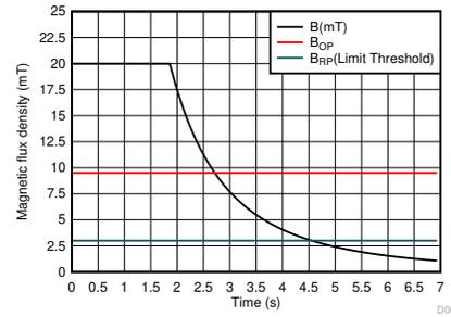
**Figure 3. Magnetic Flux Density for Case Tamper Detection**
