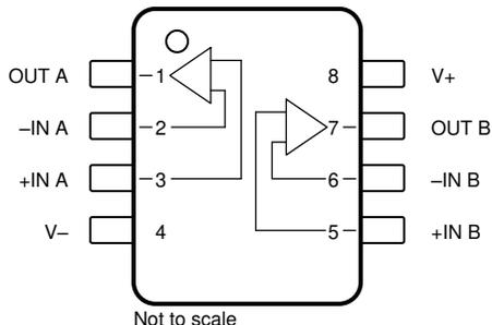
**Figure 4-2. Pin Diagram (OPA2376QDGKRQ1 (DGK) Package)**
