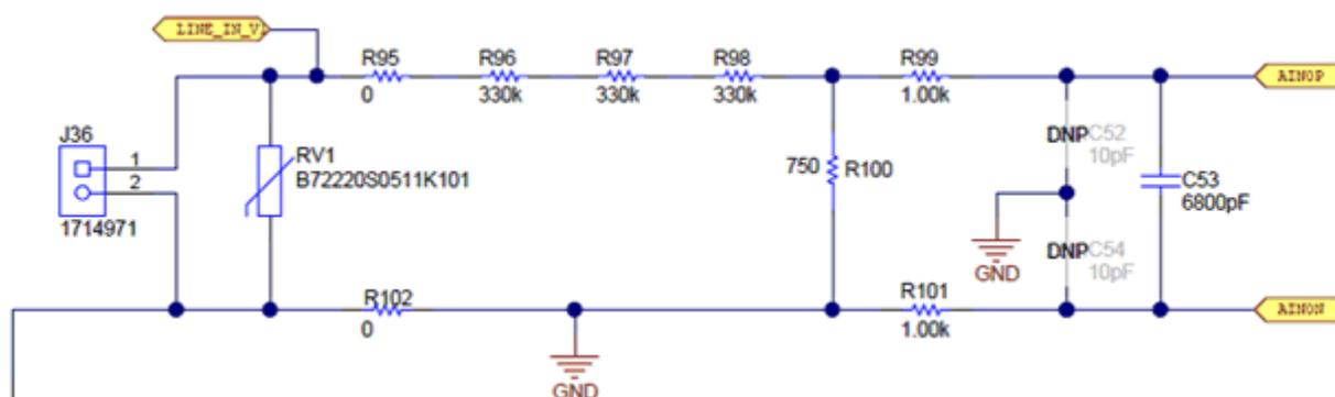
Figure 3-1. Analog Front End for Voltage Inputs
