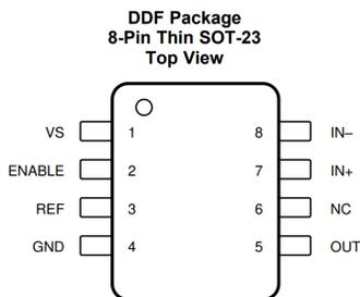
**Figure 4-2. Pin Diagram (DDF-8 Package)**
