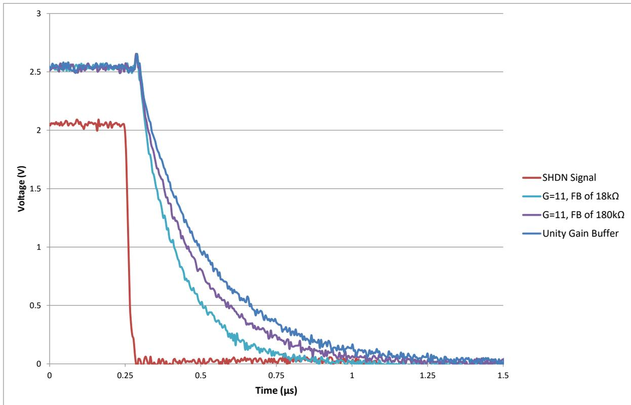
Figure 5-4. Closed-Loop Configuration and Shutdown TLV9062S
