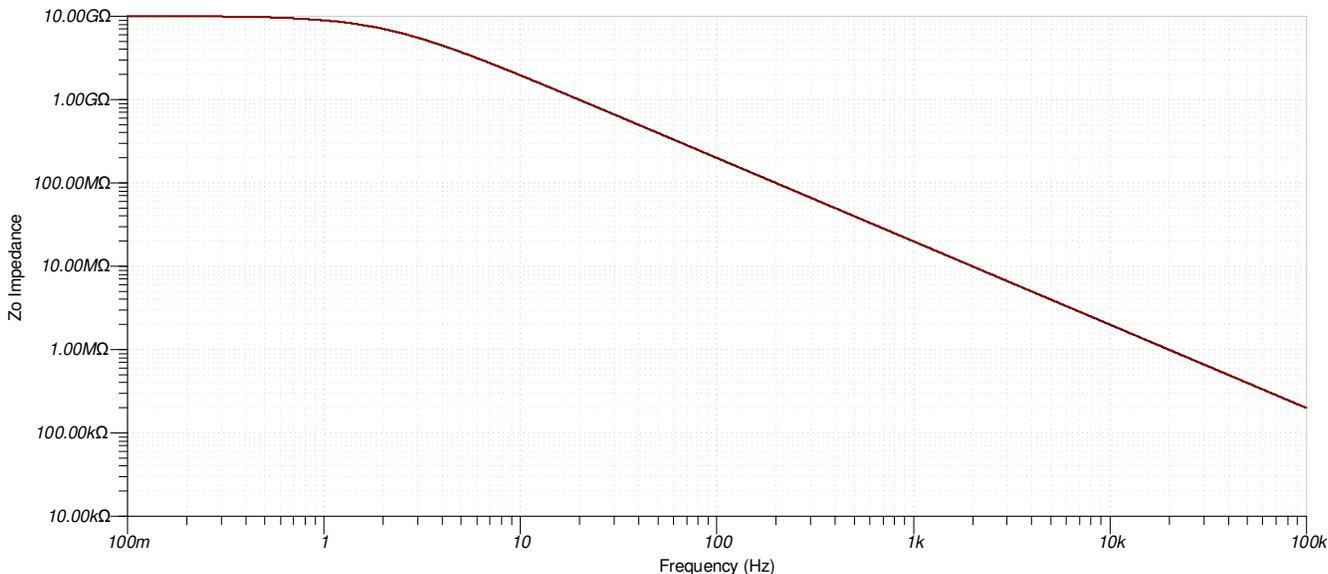
**Figure 2-2. Output Impedance During Shutdown**
