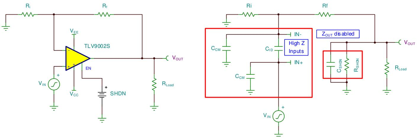
Figure 6-3. Non-Inverting Amplifier Circuit
