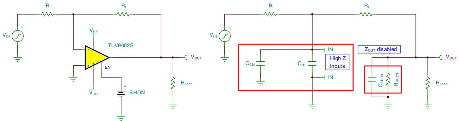
**Figure 6-1. Inverting Amplifier Circuit**
