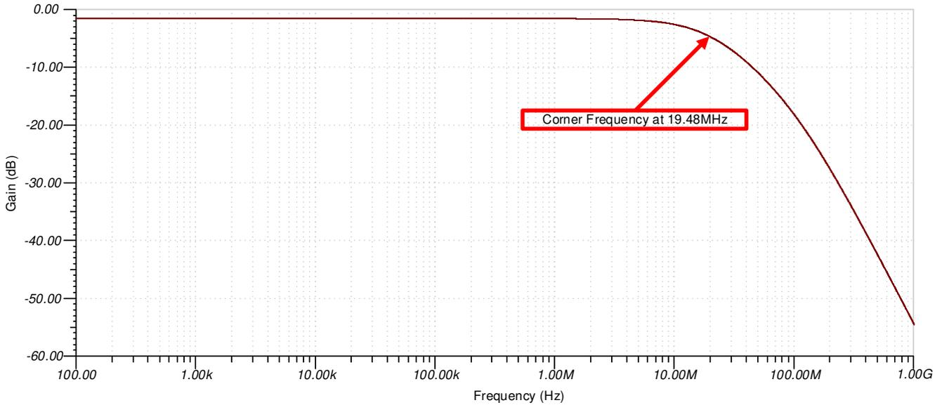
Figure 6-2. Inverting Amplifier AC Response
