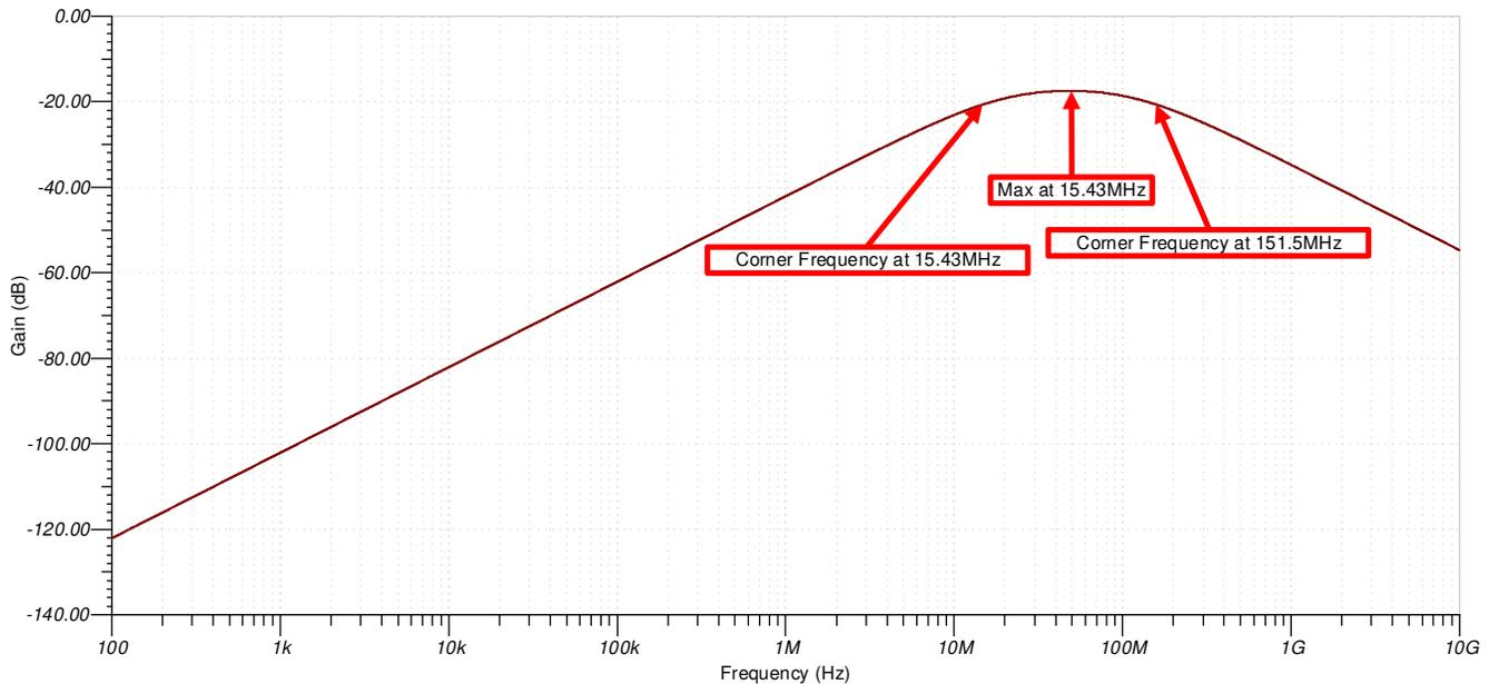
Figure 6-4. Non-Inverting Amplifier AC Response
