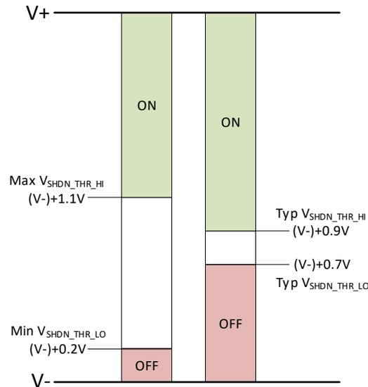
**Figure 2-3. Shutdown Threshold Graphic**
