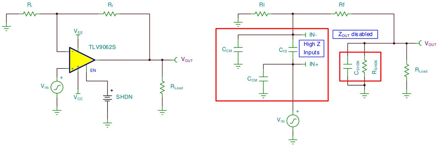
Figure 5-3. Non-Inverting Amplifier Circuit
