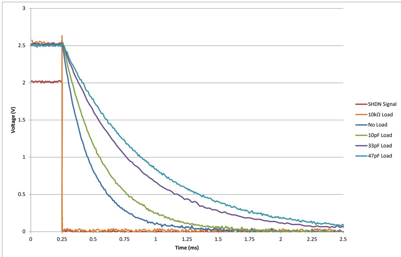
Figure 5-2. Load and Shutdown TLV9062S
