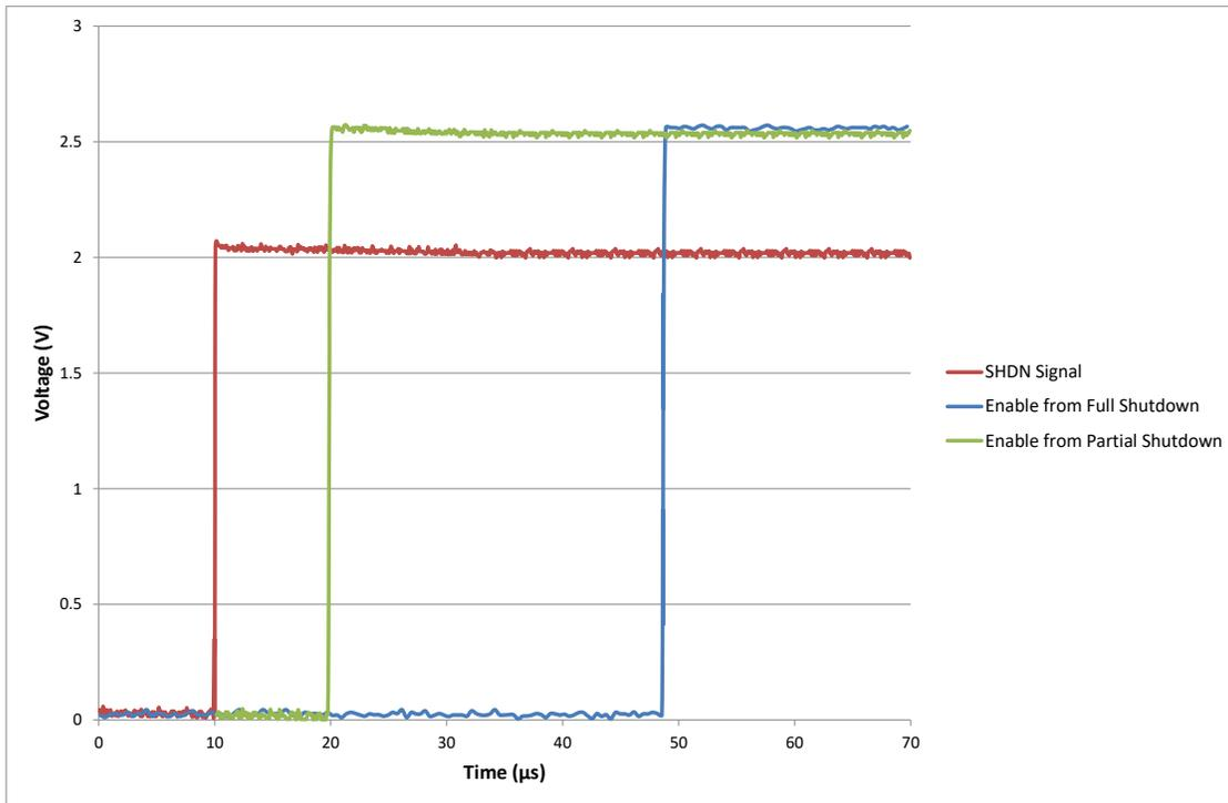
**Figure 4-1. TLV9052S Enable From Full Shutdown and From Partial Shutdown**
