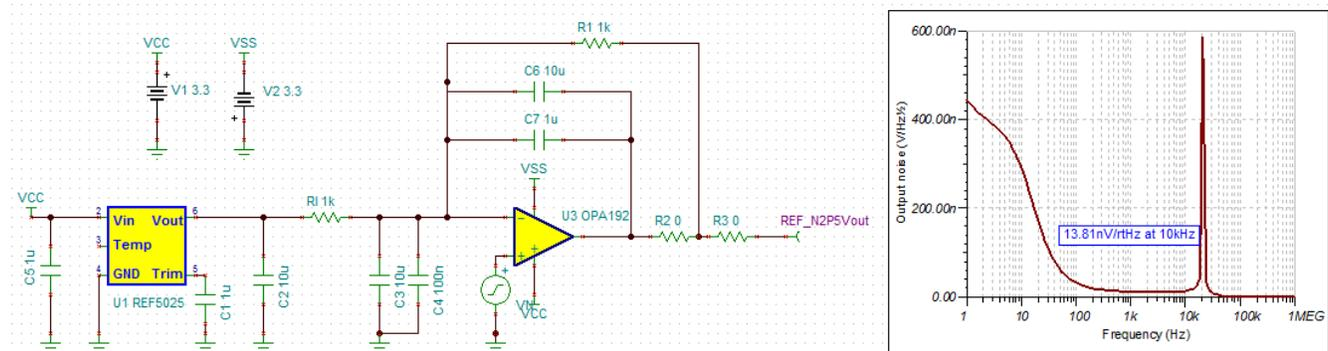
Figure 5. Adding Low-Frequency Filter to Minimize Output Noise
