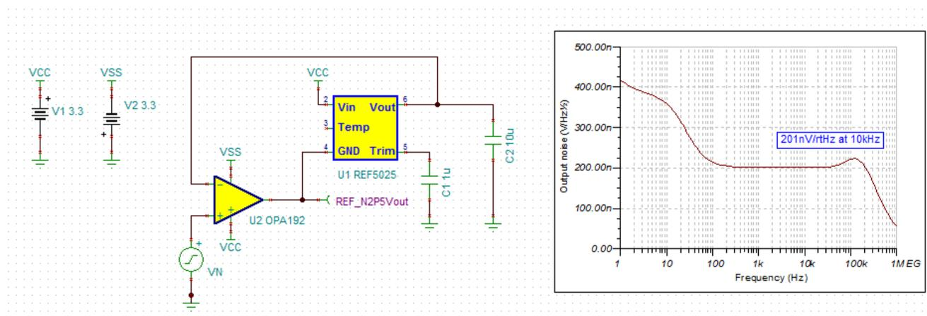
Figure 3. Level Shifting Circuit and Noise Analysis Result
