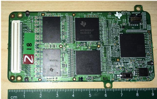
Figure 8. Transceiver Board Top View
