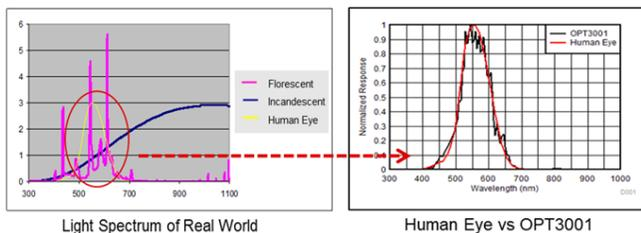
**Figure 3. [OPT3001-Q1](#) Response (Wavelength on Y-Axis)**
