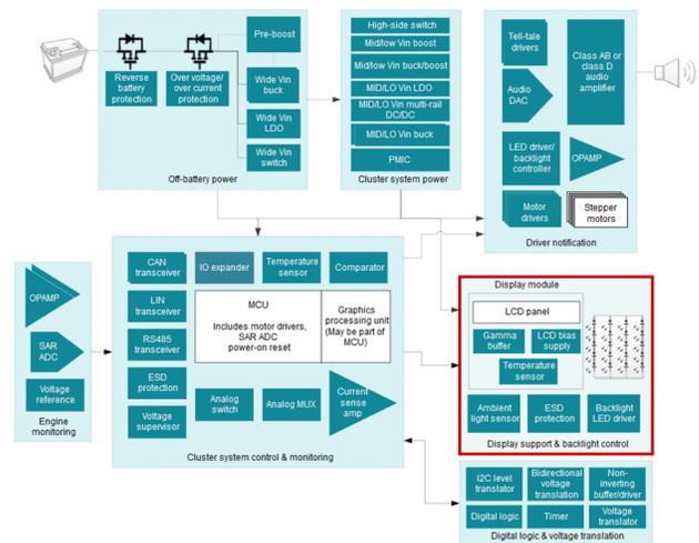
Figure 1. Cluster Block Diagram (See Other Automotive Block Diagrams on [ti.com](#))
