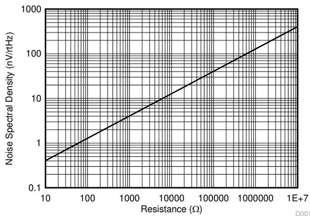
**Figure 1-1. Voltage Noise Density Curve**
