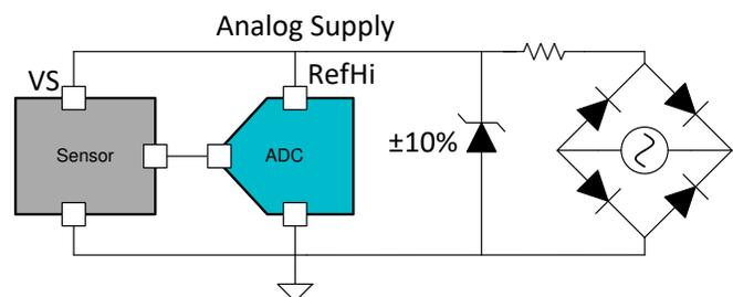
Figure 3. Ratiometric Sensor Architecture for Poorly Regulated Supplies
