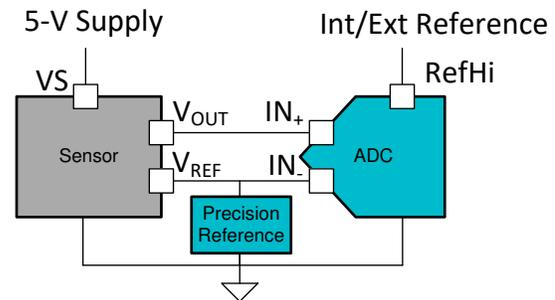
**Figure 5. TMCS1100 Optimized Signal Chain**
