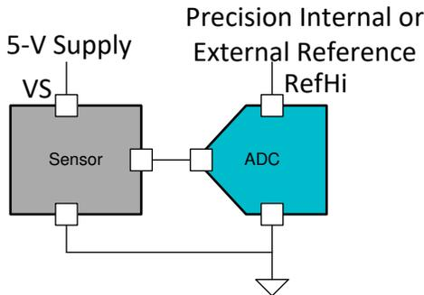
**Figure 4. Non-Ratiometric Architecture for Precision Signal Chains**
