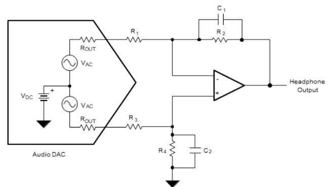
Figure 2. Audio DAC Output Circuit
