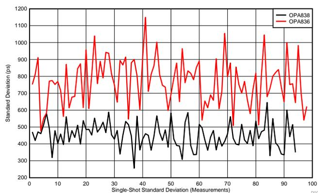
**Figure 3. 200-kHz Single-Shot Standard Deviation (STD) OPA838 vs OPA836**
