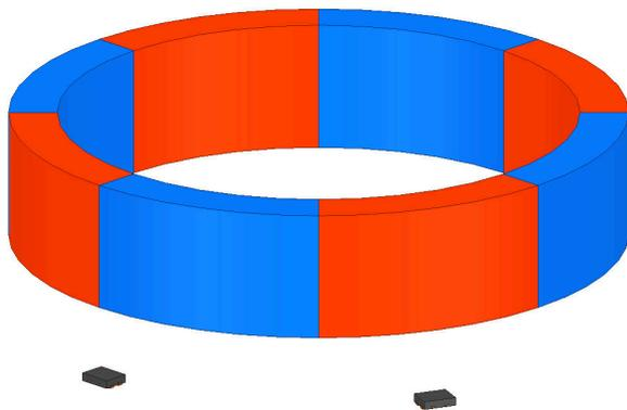
**Figure 3. Magnetic Incremental Encoder**
