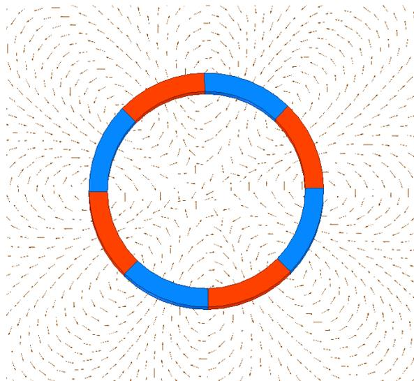
**Figure 4. In-Plane Magnet Field Vectors**
