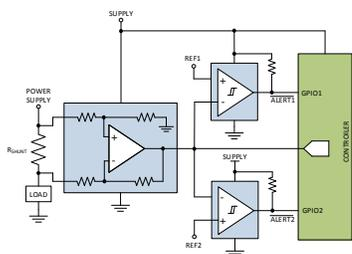
**Figure 1-1. Discrete Implementation to Detect Multiple Over-current Events**
