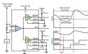
**Figure 1-3. INA303 Over and Under Current Detection**
