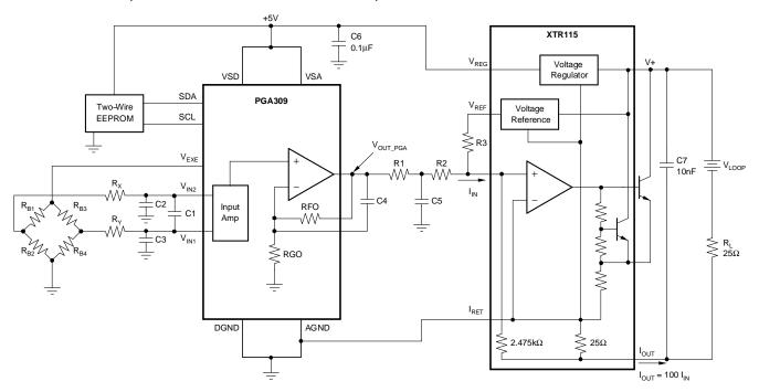
Figure 1. PGA309 and XTR115 Connections for a 4mA to 20mA Output
