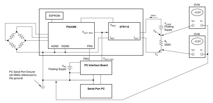
Figure 2. Power Supply and Grounding Connections for PGA309 and XTR115
