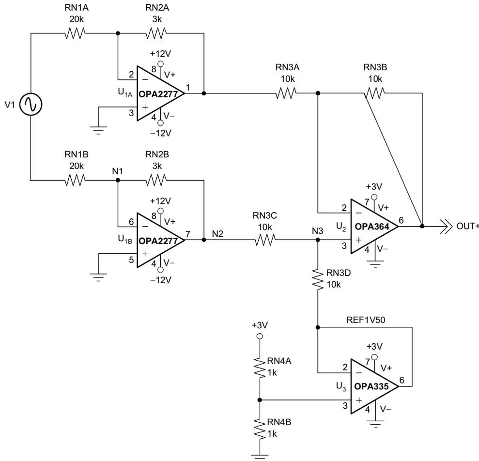
Figure 8. Circuit 5 (Circuit 1 with Differential Input)
