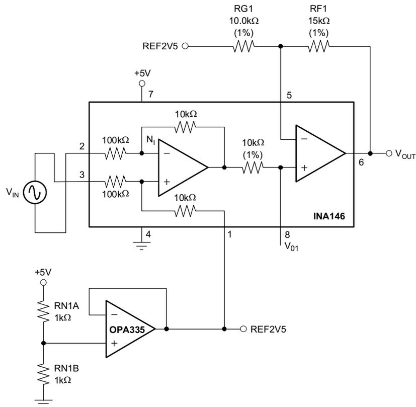
Figure 7. Circuit 4 (Circuit 3 with Differential Input)
