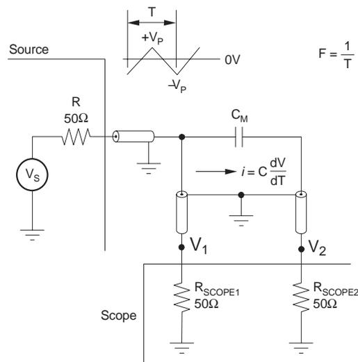
**Figure 5. Computing  $V_2$  for Triangle Wave  $V_1$**
