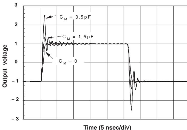
Figure 3. Time-Domain Plot for Current Feedback Amplifier
