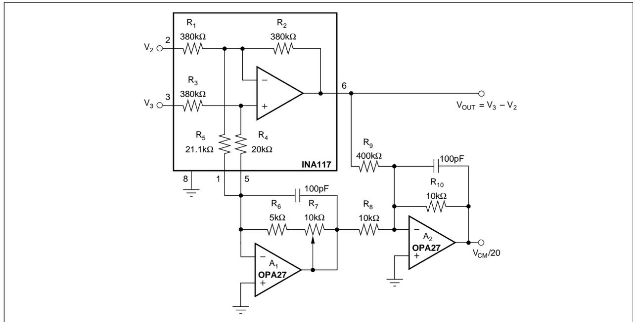
FIGURE 2. INA117 with True Common-Mode Voltage Monitor.
