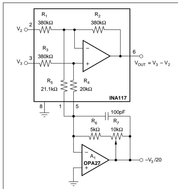
FIGURE 1. INA117 with V<sub>3</sub> Common-Mode Voltage Monitor.
