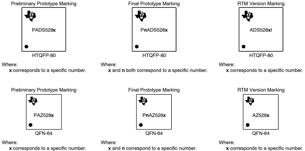
This document describes the planned record of revisions to the design of the ADS528x family with respect to the *preliminary prototype version* of the silicon that is being sampled in Q1, 2007. The next version of silicon (referred to in these errata as the *final prototype*) incorporates all the corrections listed in these errata. These corrections will also be reflected in the RTM version of the product data sheet.
