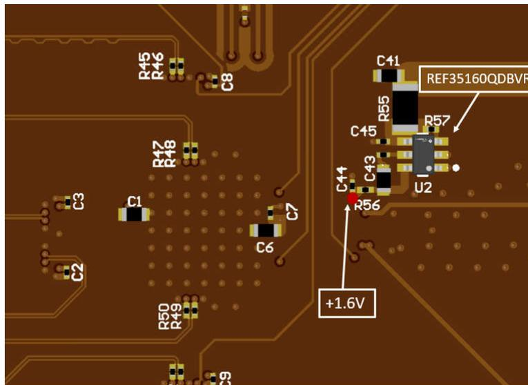
Figure 3-2. ADC36xxEVMCVL Features Identification (Bottom)
