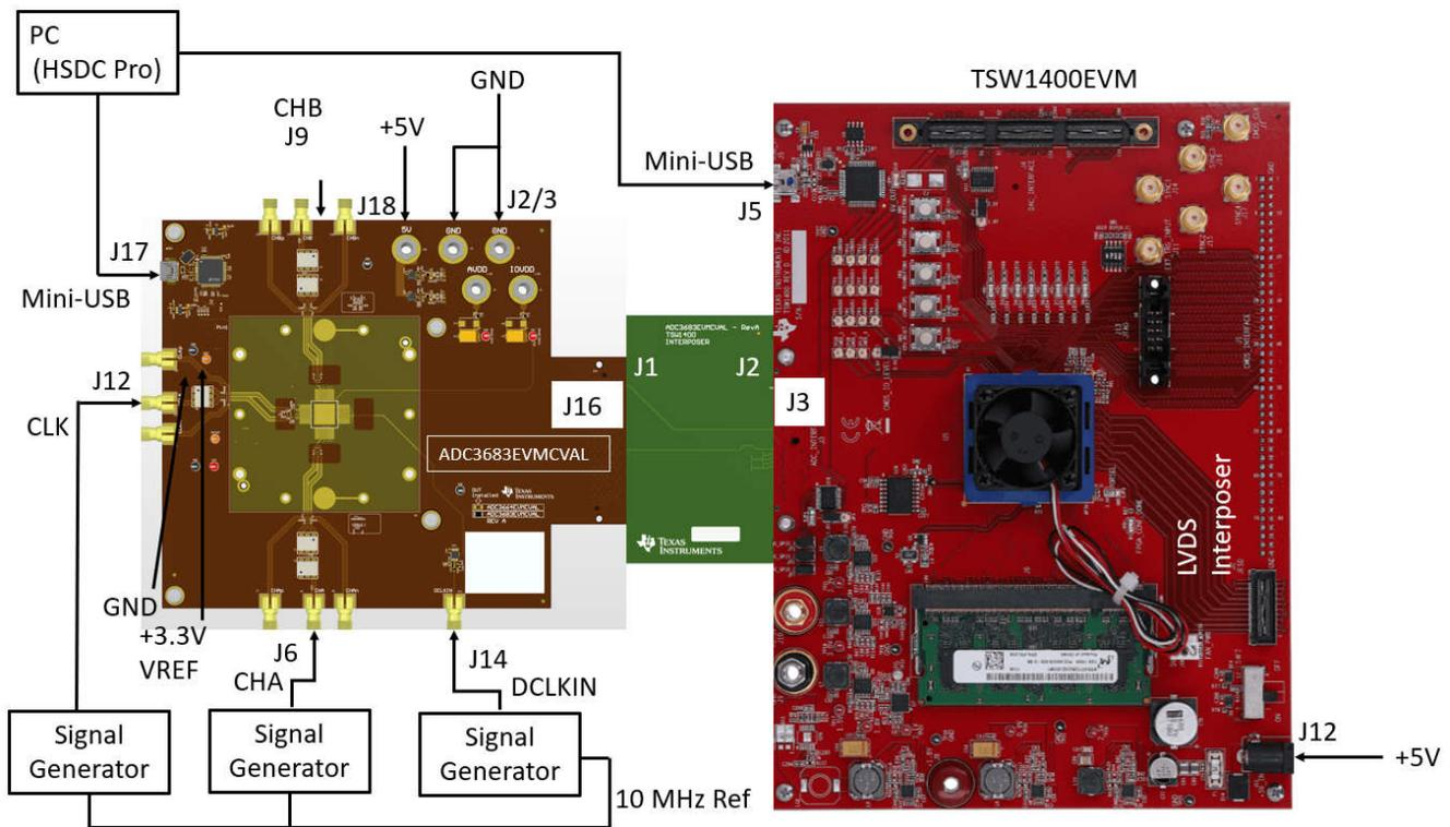
Figure 1-1. ADC36xxEVMCVAL Block Diagram
