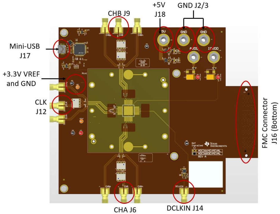
Figure 3-1. ADC36xxEVMCVL Features Identification (Top)
