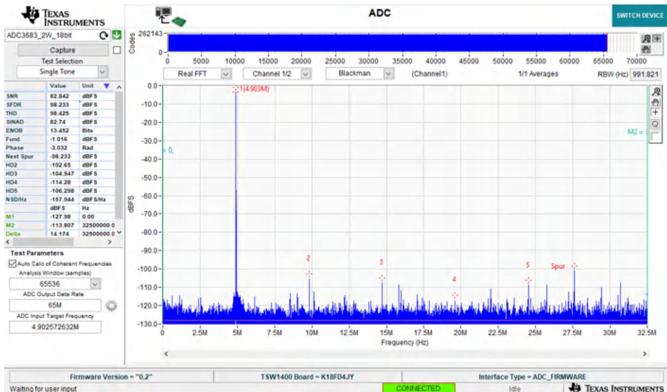
Figure 4-3. ADC36xxEVMCVAl Default Configuration Capture
