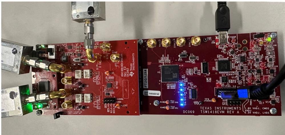
**Figure 2-3. Final Setup of ADC3910D125EVM**
