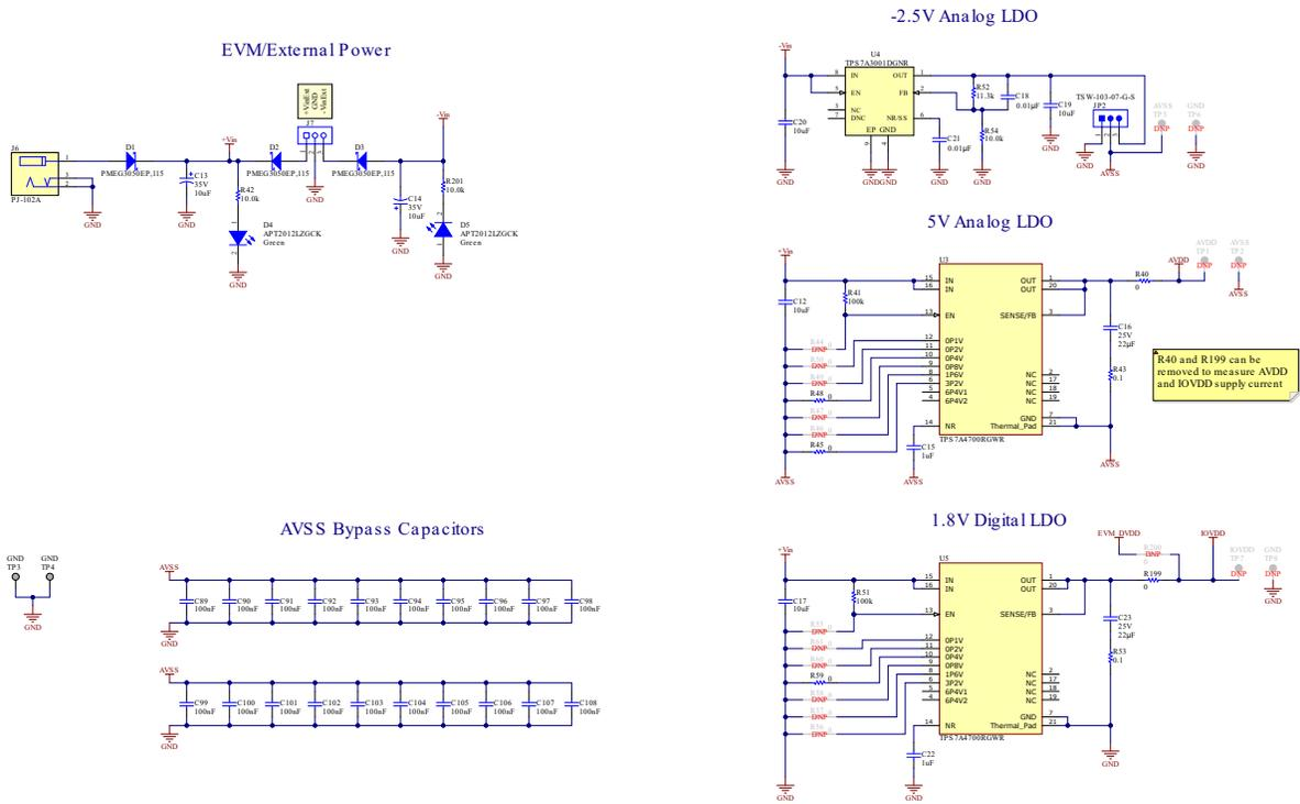
Figure 5-2. ADS127L18EVM External Power Schematic
