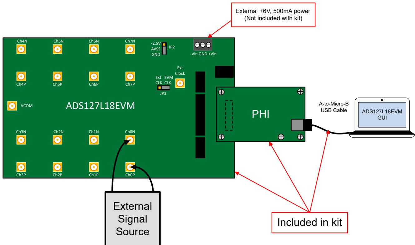
**Figure 1-1. System Connection for Evaluation**
