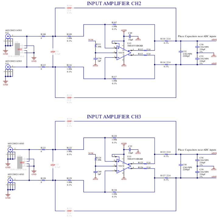
Figure 5-5. ADS127L18EVM Input Channels 2 and 3 Schematic
