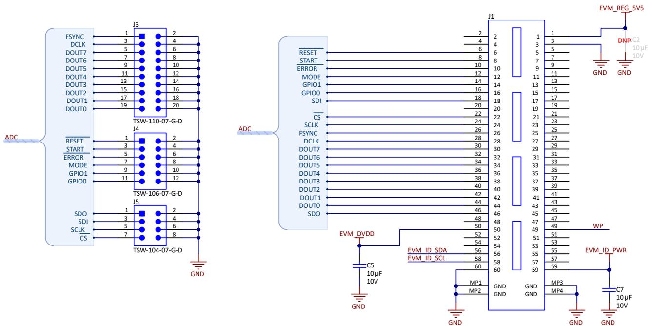
Figure 2-9. Connections to Digital Signals on PHI and Test Points
