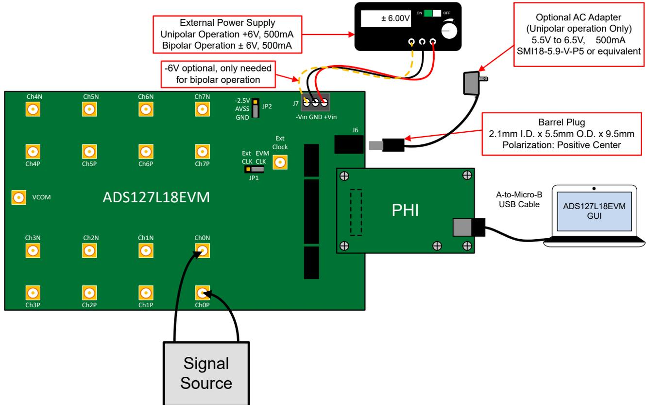
Figure 2-2. Power Connections
