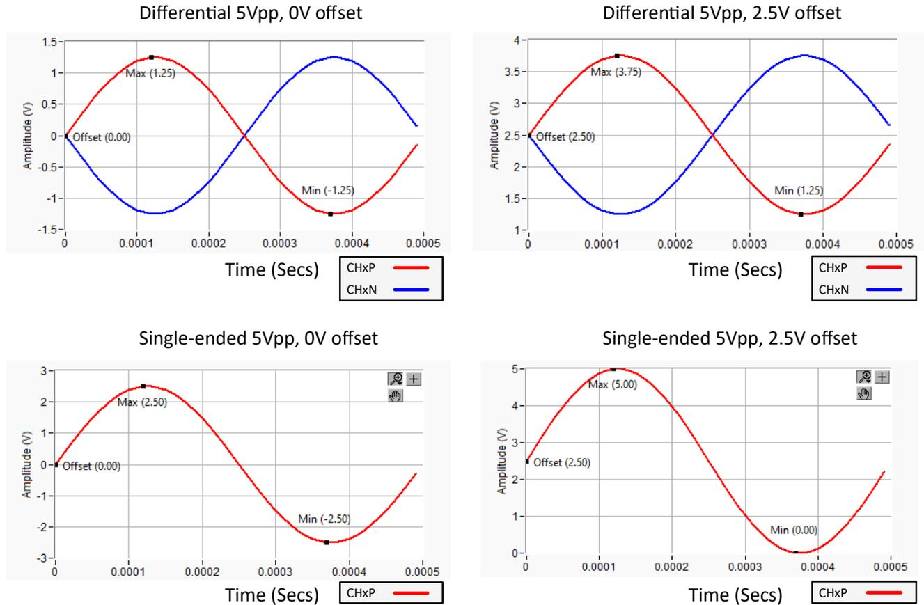
Figure 2-1. Maximum input signal range (Vref = 2.5V)
