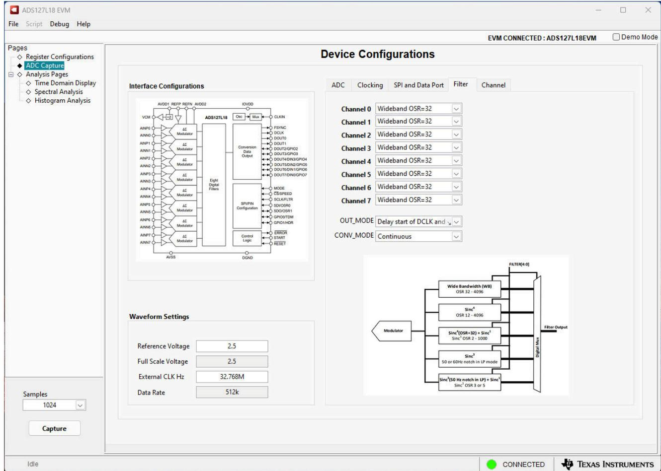
The screenshot displays the 'Device Configurations' window for the ADS127L18 EVM. The 'Filter' tab is active, showing configuration options for 8 channels. The 'Channel 0' through 'Channel 7' dropdowns are all set to 'Wideband OSR=32'. Other settings include 'OUT\_MODE' set to 'Delay start of DCLK and...' and 'CONV\_MODE' set to 'Continuous'.
