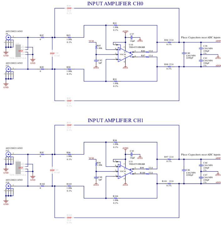
Figure 5-4. ADS127L18EVM Input Channels 0 and 1 Schematic
