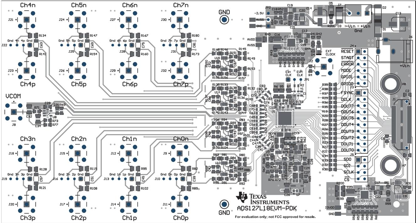
Figure 5-8. PCB Layout for the ADS127L18EVM (Top View)
