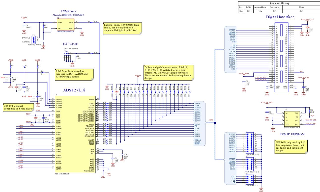
Figure 5-1. ADS127L18EVM ADC Interface and Reference Schematic
