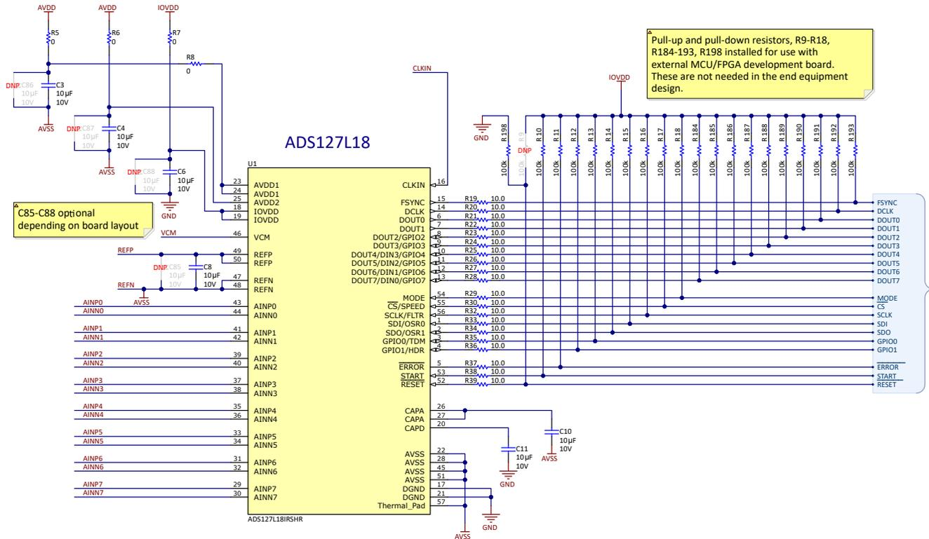
Figure 2-3. ADS127L18 Connections and Decoupling
