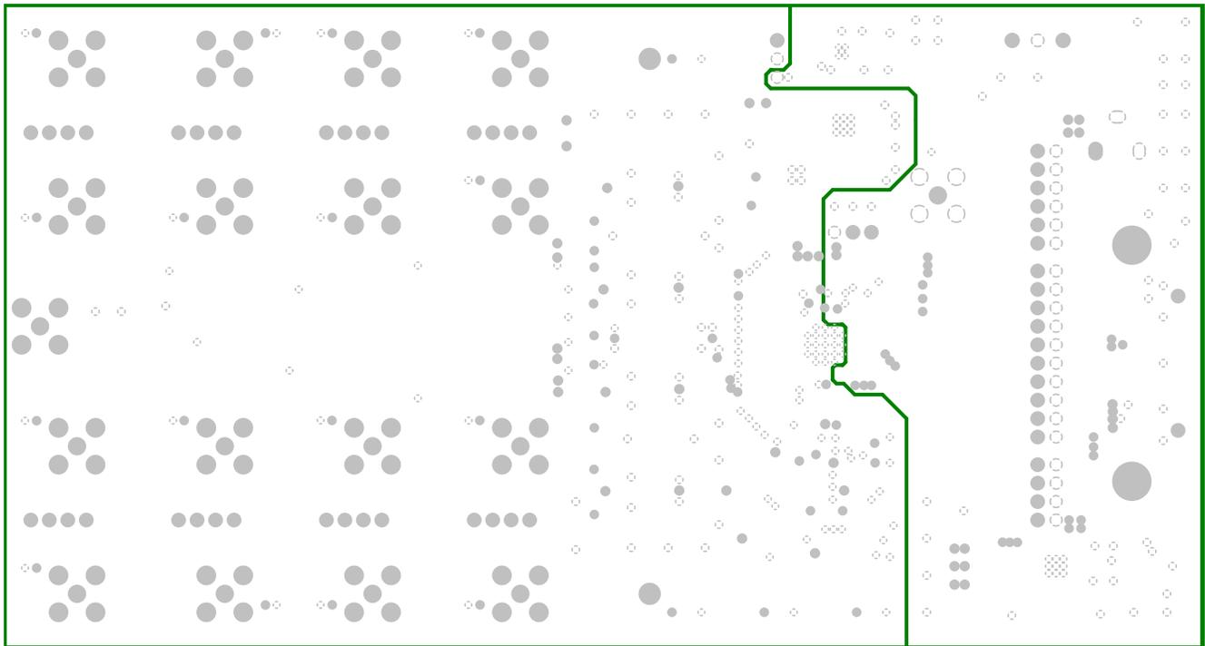
**Figure 5-10. PCB Layout (internal AVSS/GND plane 1) for the ADS127L18EVM**
