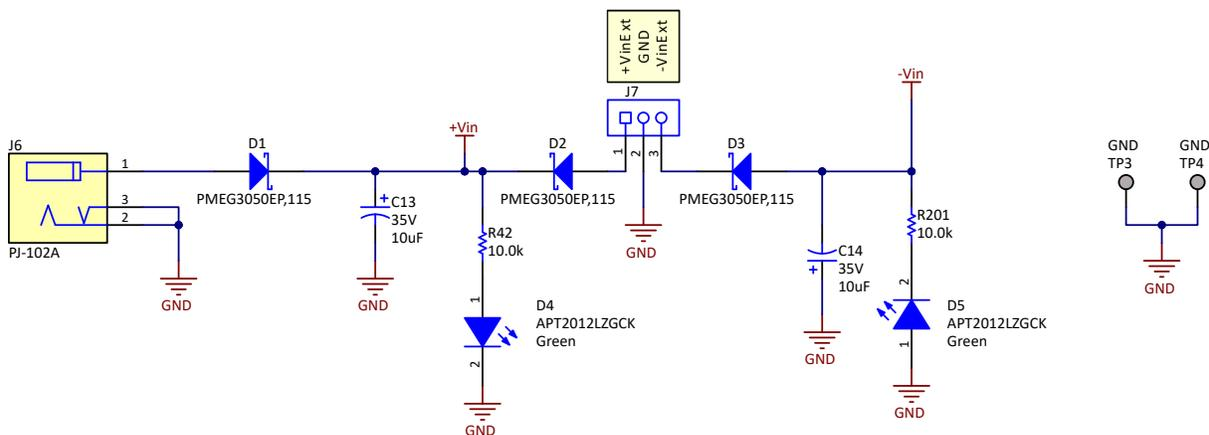
Figure 2-11. External Power Supply Connections
