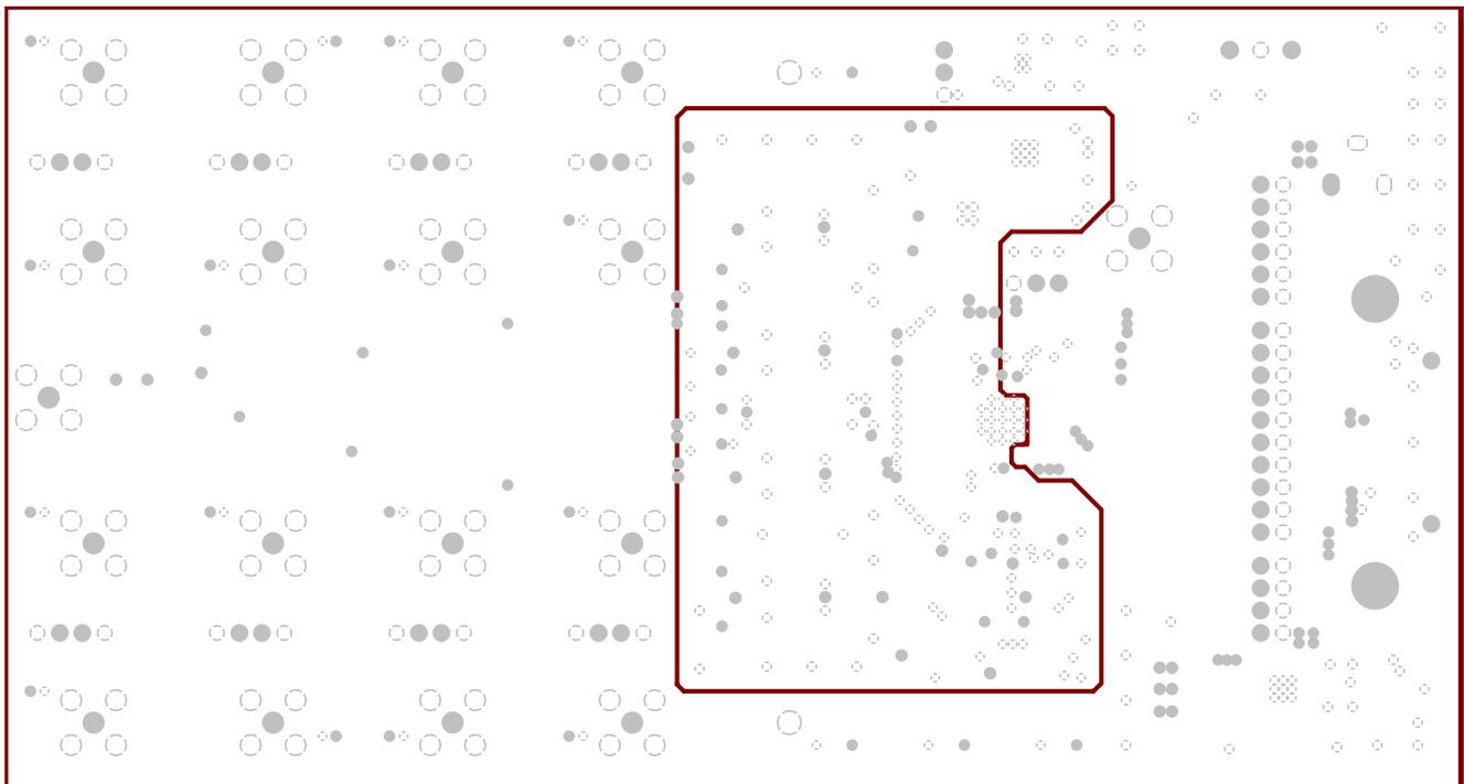
**Figure 5-11. PCB Layout (internal AVSS/GND plane 2) for the ADS127L18EVM**
