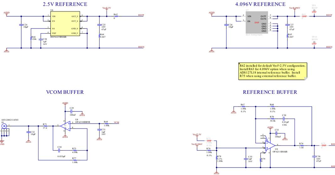
Figure 5-3. ADS127L18EVM Reference and VCOM Buffer Schematic
