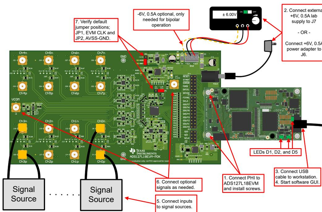
Figure 4-1. Connecting the Hardware to the ADS127L18EVM
