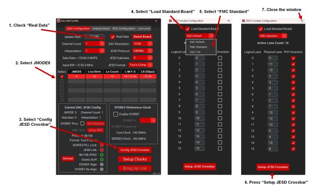
Figure 2-4. DAC39RF12EVM GUI Configuration, Part 1
