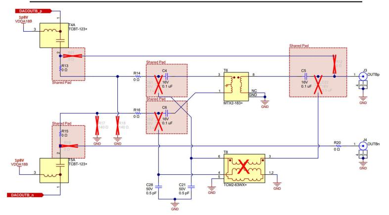
A. DACB Output stage. By default the MTX2-183+ balun is used for this channel. (2MHz to 18GHz)
