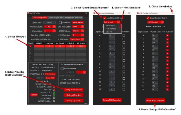
Figure 2-9. DAC39RF12EVM GUI Configuration, Step 1
