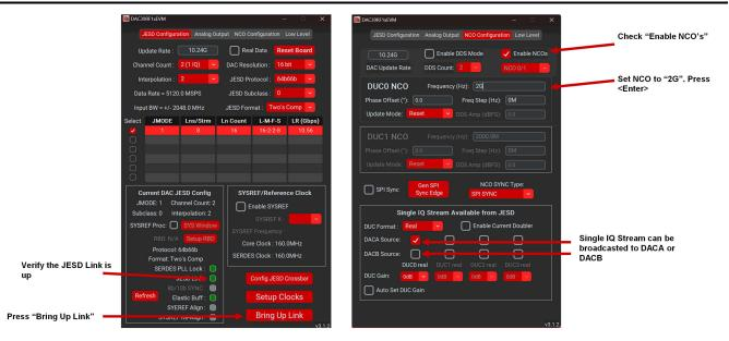
Figure 2-12. DAC39RF12EVM GUI Configuration Steps, Step 4: Moving the modulated waveform up in frequency.
