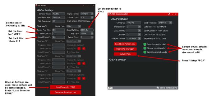
Figure 2-11. DAC Wavegen GUI & J59 Commander setup details, Step 3
