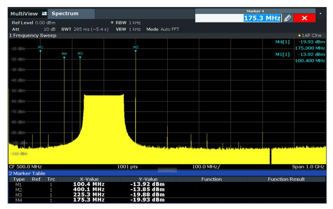
Figure 2-19. DAC39RF12EVM, CHA Output Spectrum in JMODE 3, Baseband Data
