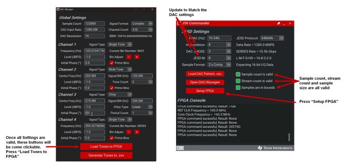
Figure 2-17. DAC Wavegen GUI & J59 Commander setup details, Step 3
