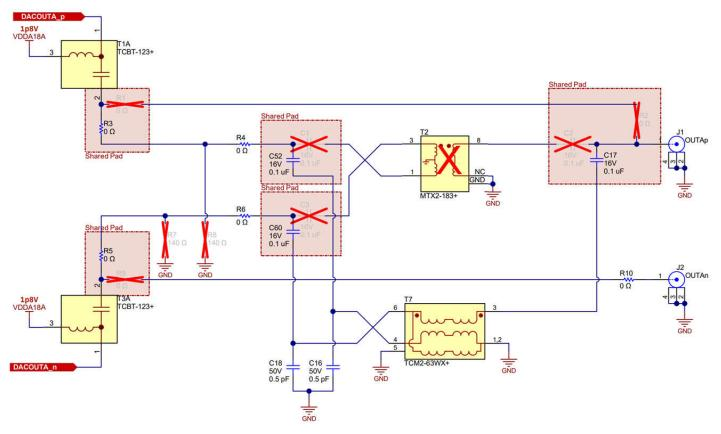
A. DACA Output stage. By default the TCM2-63WX+ balun is used for this channel. (30MHz to 6GHz)
