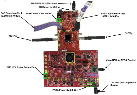
Figure 2-1. DAC39RF12EVM Test Setup
