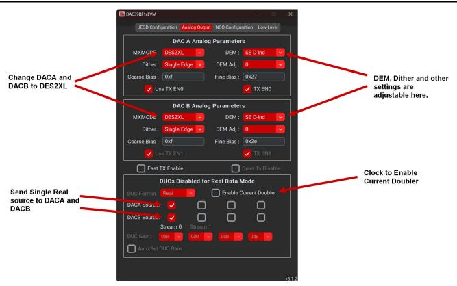
Figure 2-7. DAC39RF12EVM GUI Configuration Steps, Step 4
