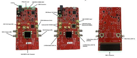
Figure 1-1. DAC39RF12EVM Key Components
