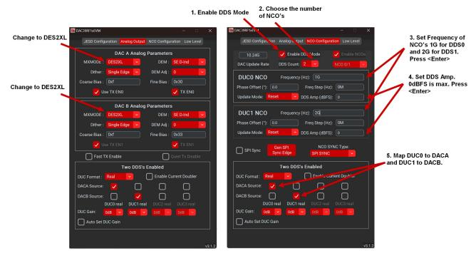
Figure 2-22. DAC39RF12EVM GUI Configuration for DDS Mode
