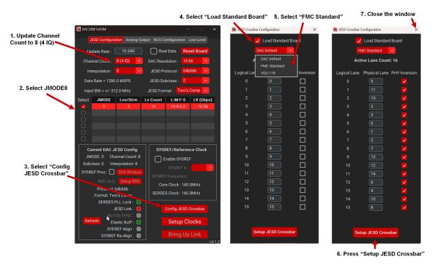
Figure 2-15. DAC39RF12EVM GUI Configuration, Step 1
