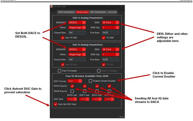
Figure 2-18. DAC39RF12EVM GUI Configuration Steps, Step 4
