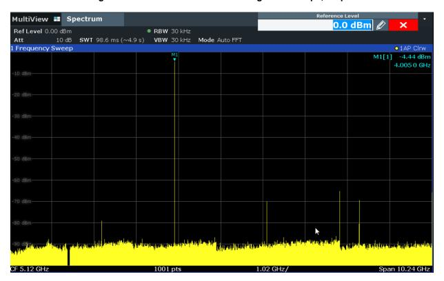
Figure 2-8. DAC39RF12EVM, CHA Output Spectrum in JMODE 0, DES2XL Mode
