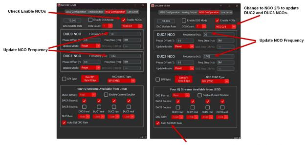
Enable this to prevent oversaturation. Each DUC is lowered by 12dB as they are summed.
