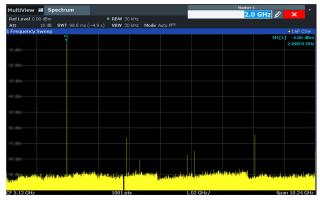
DACB Generating a 2GHz tone in DDS mode. Note the reduced  $2^{\rm nd}$  Nyquist image due to DES2XL output mode
