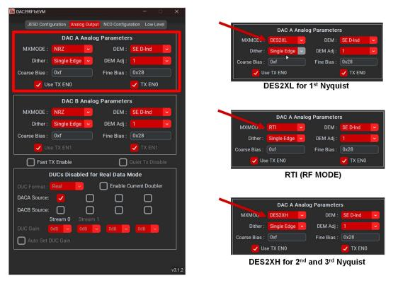
Figure 2-13. DAC39RF12EVM GUI Configuration Steps, Step 5
