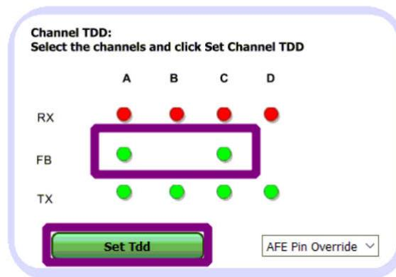
Figure 4-21. TDD Configuration for TX to FB Test
