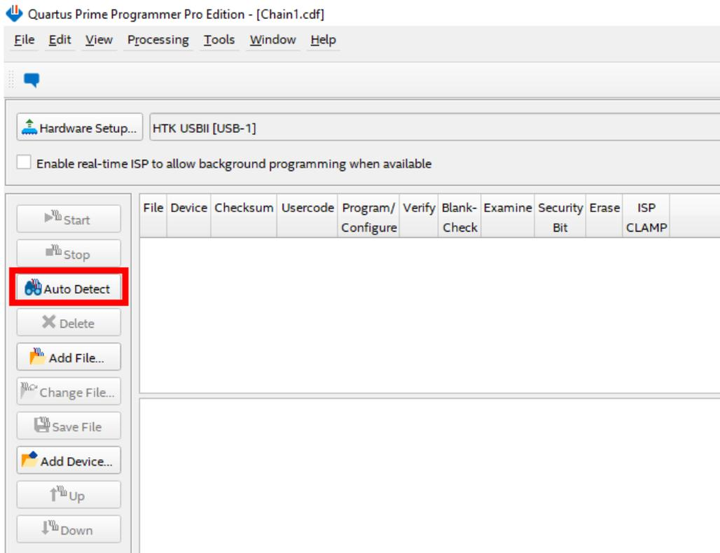
**Figure 4-8. Auto Detect in Quartus Prime Programmer**
