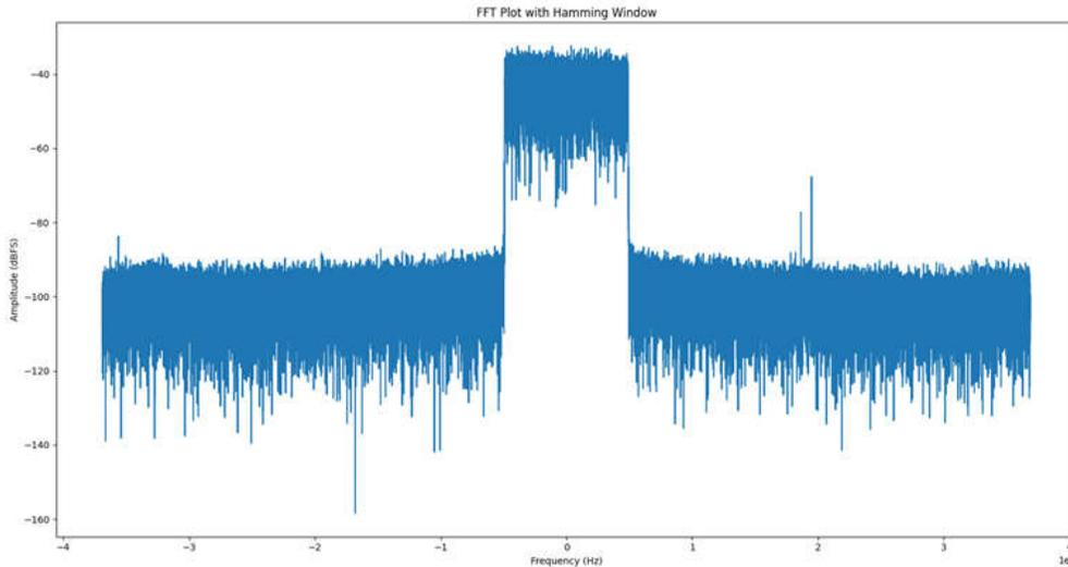
**Figure 5-2. FFT Showing the Loop-Backed TM3.1a Waveform**
