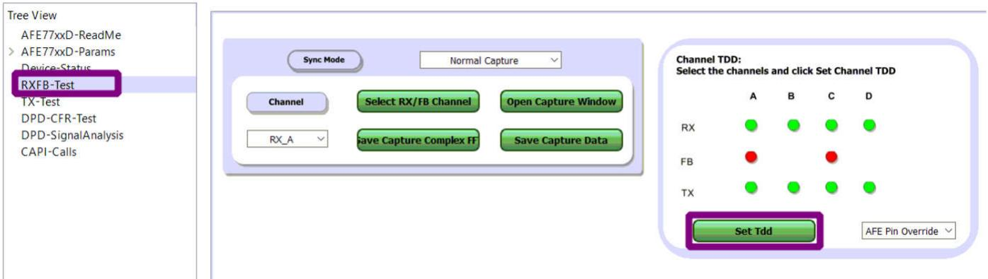
Figure 4-20. TDD Configuration for TX to RX Test
