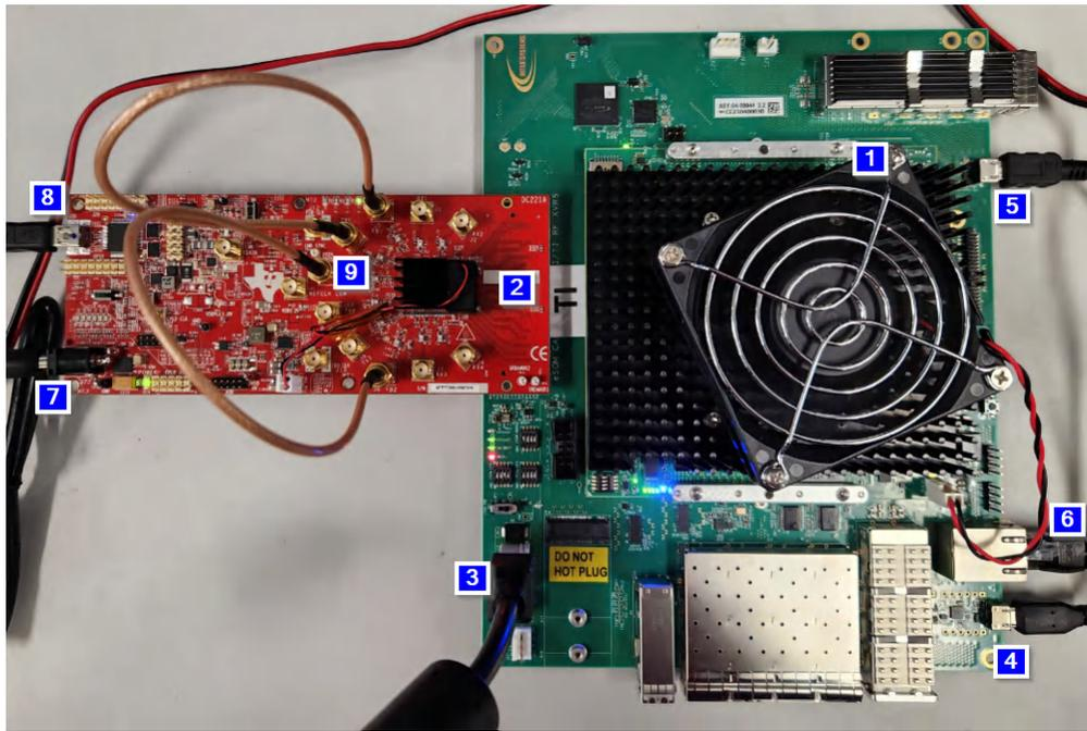
Figure 2-1. Hardware Setup, AFE7769DEVM and Agilex eSOM7
