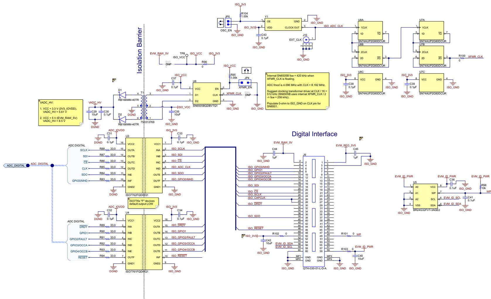
Figure 7-8. Digital Isolators, DC/DC Power Supply, External Clock, and PHI Controller
