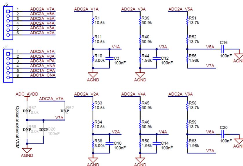
Figure 2-2. ADC2A Sequencer Input Circuits (Schematic)
