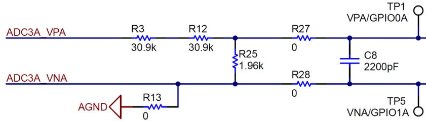
**Figure 2-3. ADC3A Voltage Input Circuit (Schematic)**
