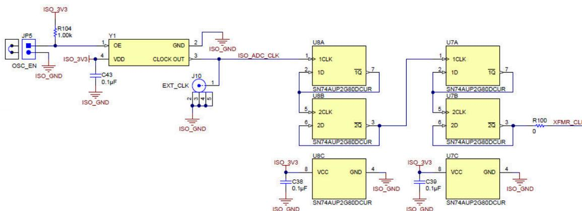
**Figure 3-1. External ADC Clock Options (Schematic)**
