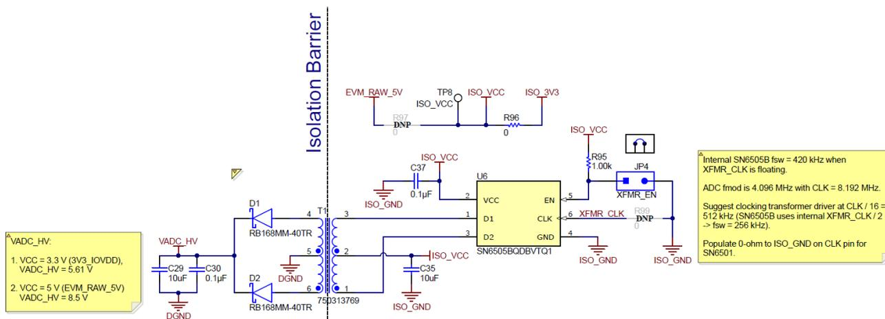
**Figure 4-1. DC/DC Converter and Transformer Driver Circuit (Schematic)**
