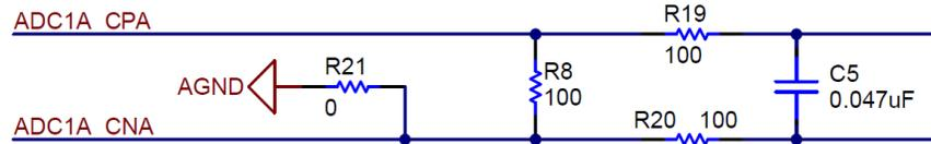
Figure 2-1. ADC1A Current Input Circuit (Schematic)
