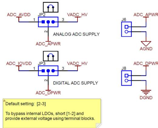
**Figure 4-2. ADC Analog and Digital Supply Options (Schematic)**
