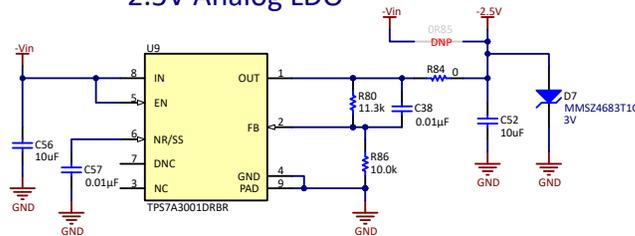
Figure 4-2. LDO Regulators for 5 V and  $-2.5$  V
