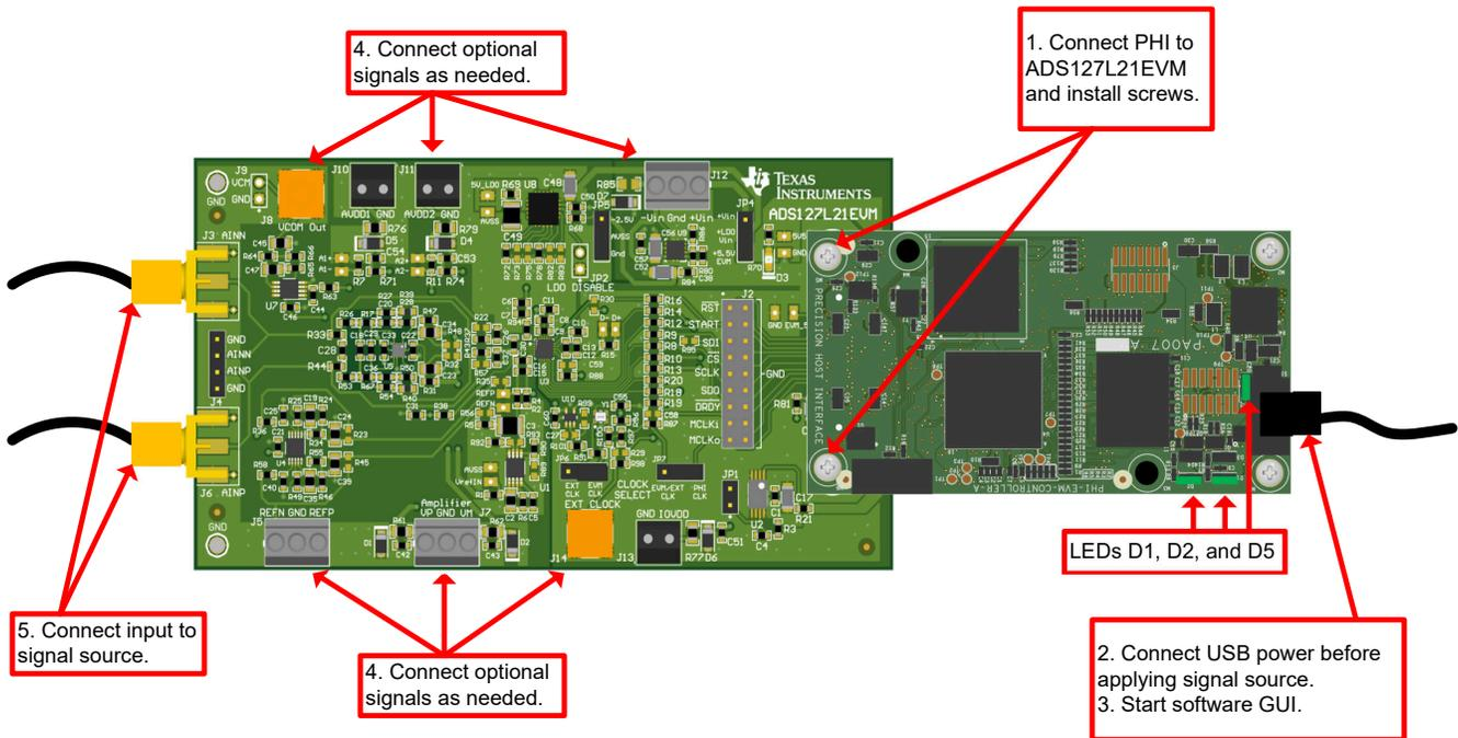
**Figure 6-1. Connecting the Hardware to the ADS127L21EVM**
