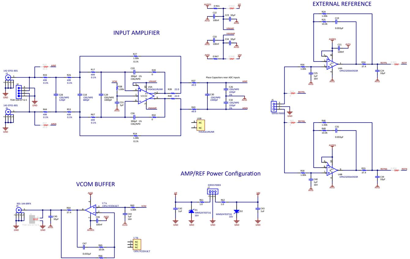
Figure 7-2. ADS127L21EVM External Reference Schematic for Input and VCOM Amplifiers
