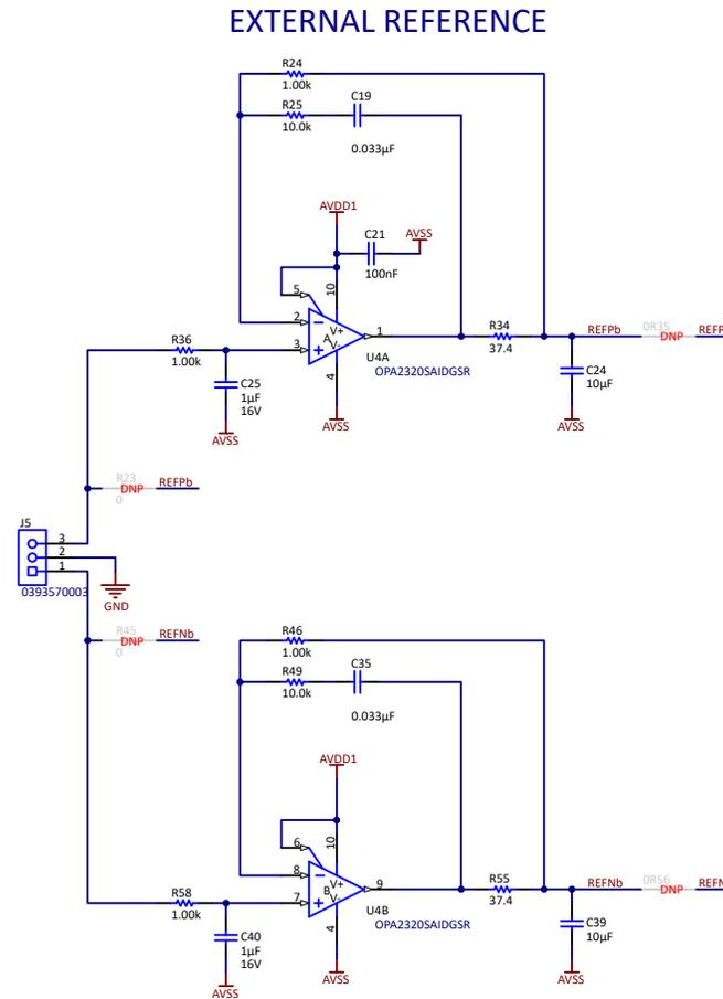
Figure 2-5. External Reference Connection and Buffer
