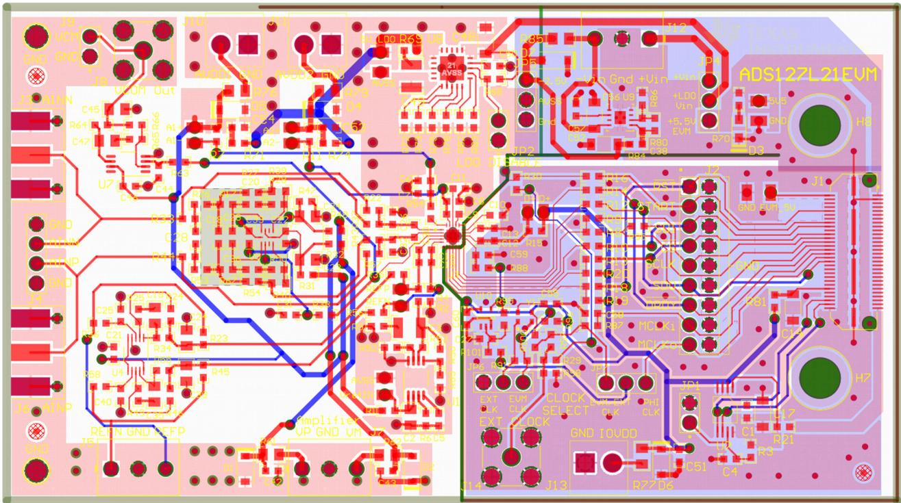
Figure 7-4. PCB Layout for the ADS127L21EVM
