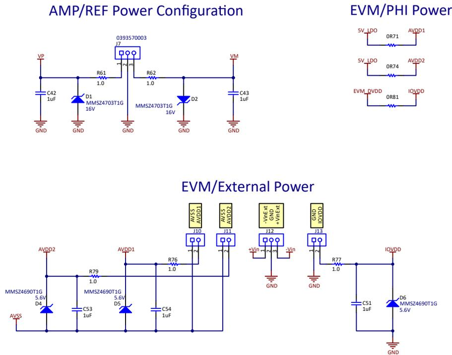
Figure 4-1. Power Connection and Configuration
