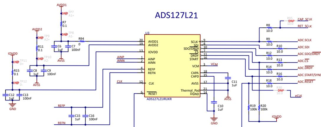
Figure 2-1. ADS127L21 Connections and Decoupling
