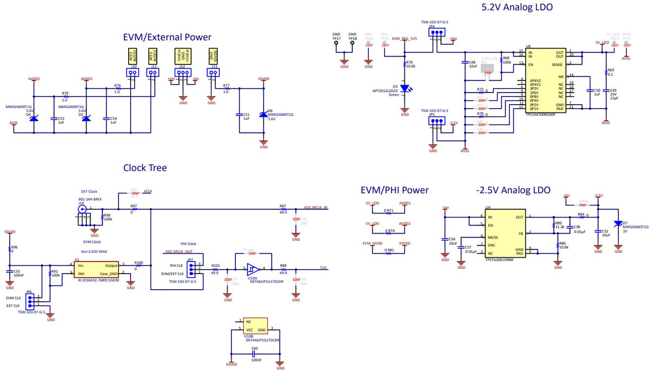
**Figure 7-3. ADS127L21EVM Clock Tree and Power Schematic**
