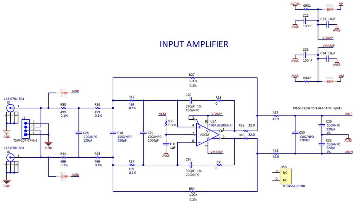
**Figure 2-2. ADC Drive Amplifier**
