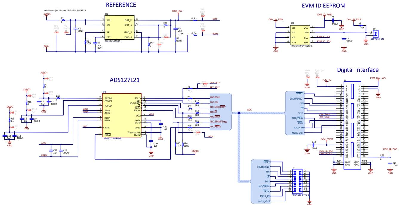
Figure 7-1. ADS127L21EVM ADC Connections and Reference Schematic
