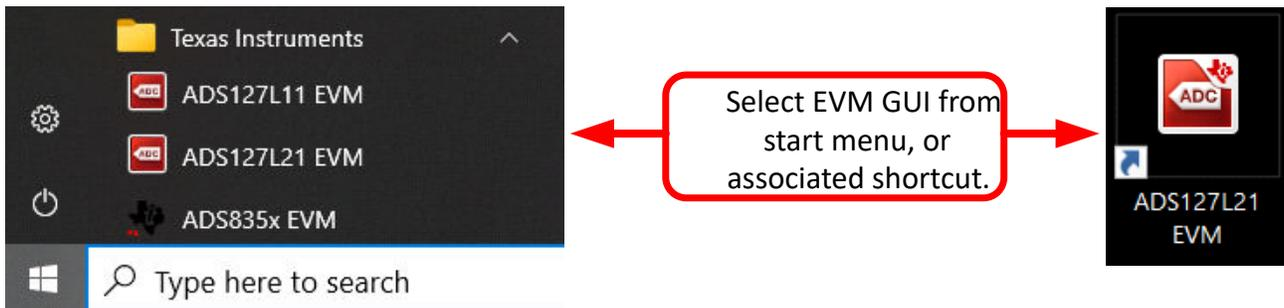
**Figure 6-2. Launch the EVM GUI Software**
