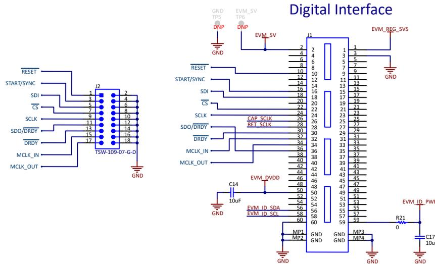
Figure 3-1. Connections to Digital Signals on PHI and Test Points
