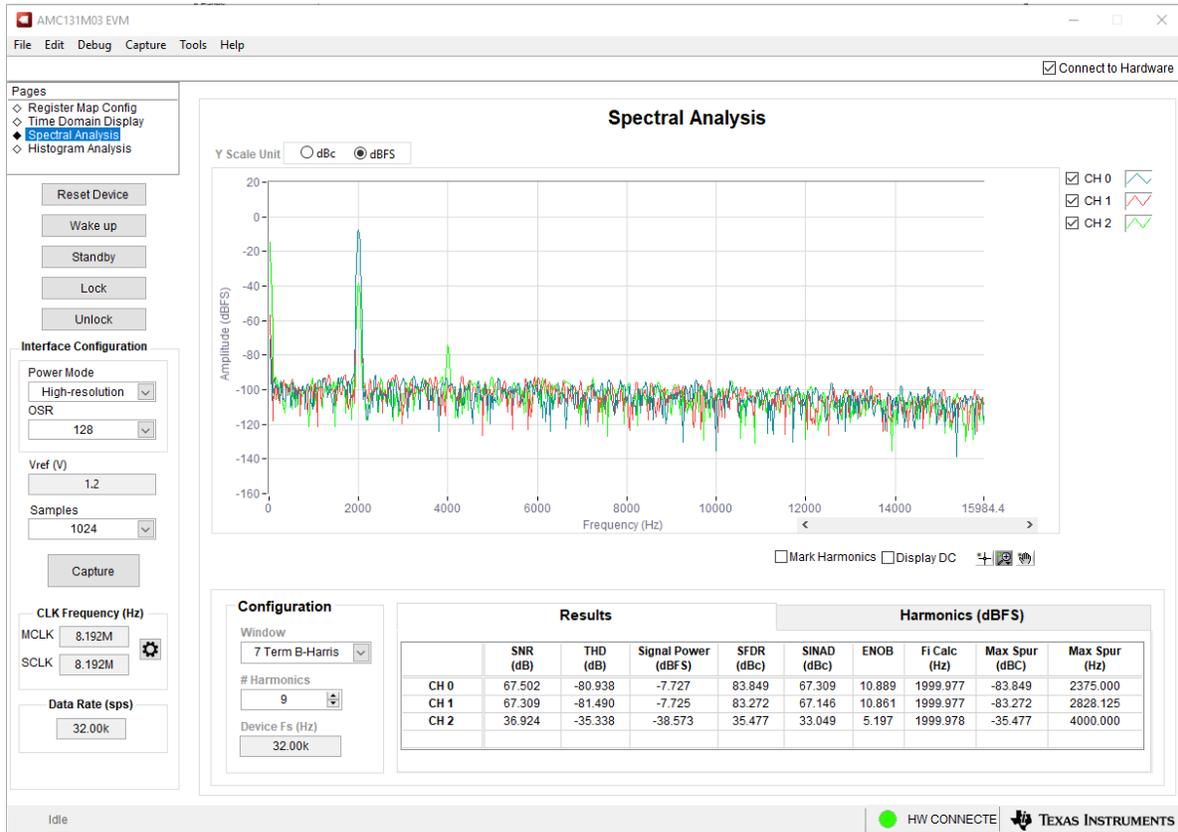
**Figure 6-7. Spectral Analysis Tool**
