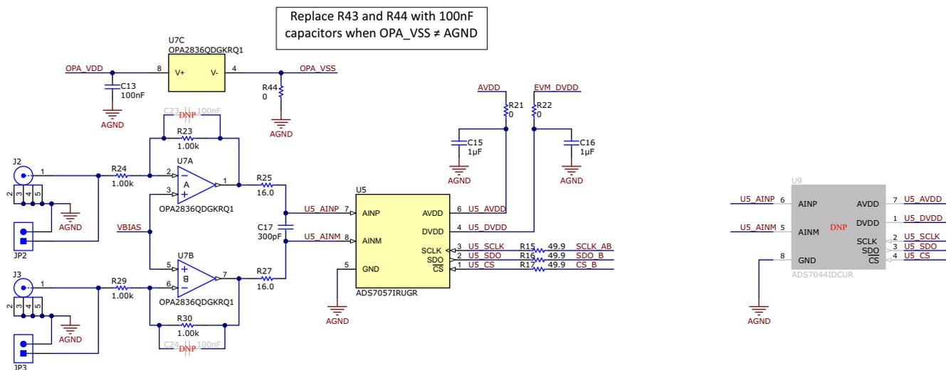
**Figure 2-3. Differential Input Path on the ADS704X-5XEVM**
