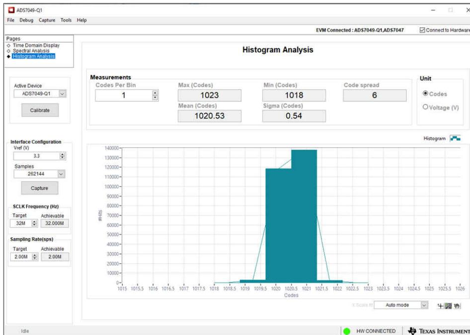
Figure 4-5. Histogram Analysis in the ADS704X-5XEVM GUI
