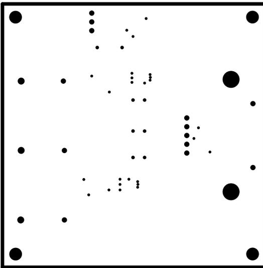
**Figure 5-4. Inner Ground Plane 1**
