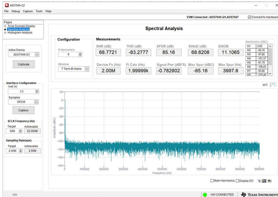
**Figure 4-4. Spectral Analysis in the ADS704X-5XEVM GUI**
