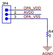
**Figure 2-5. External Power-Supply Header on the ADS704X-5XEVM**
