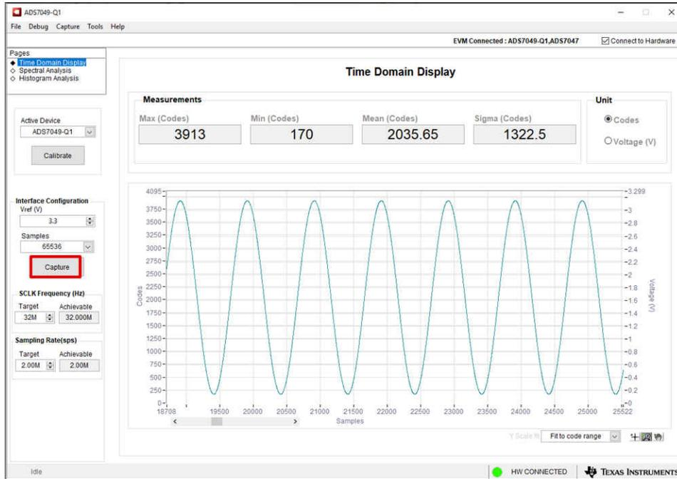
Figure 4-3. Time Domain Display in the ADS704X-5XEVM GUI
