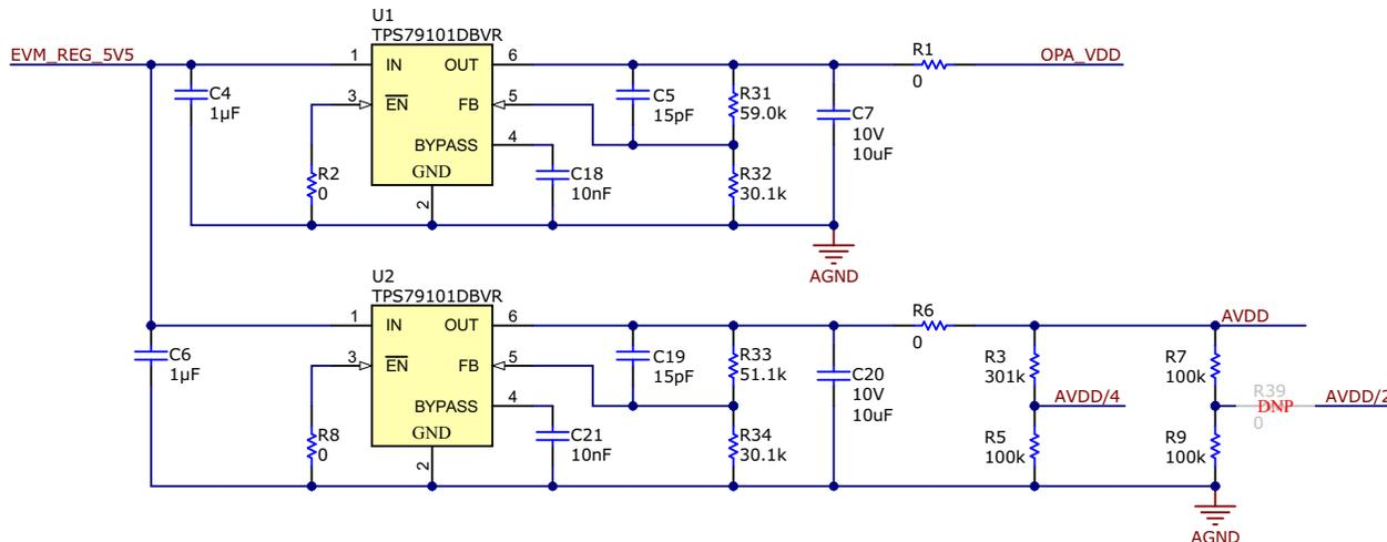
**Figure 2-4. Power Tree on the ADS704X-5XEVM**
