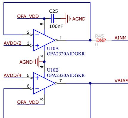
**Figure 2-6. Buffer Amplifier Circuit on the ADS704X-5XEVM**
