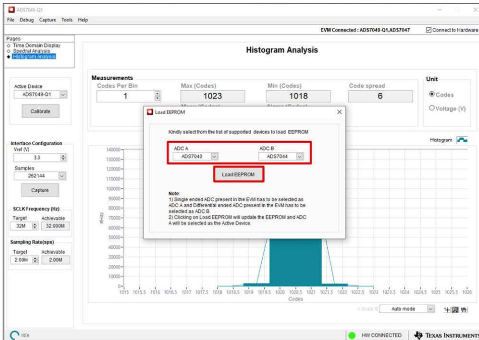
Figure 4-6. Selecting the ADCs and Loading the EEPROM
