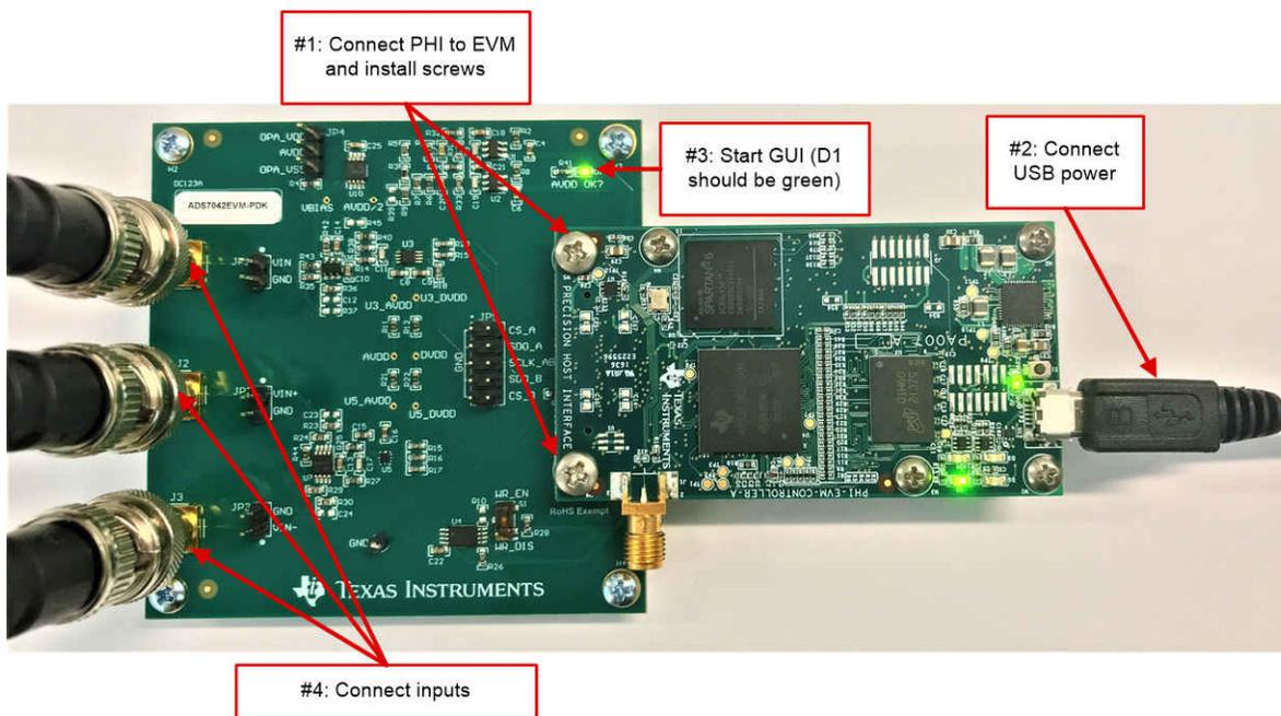
**Figure 4-1. Hardware Connections on the ADS704X-5XEVM**
