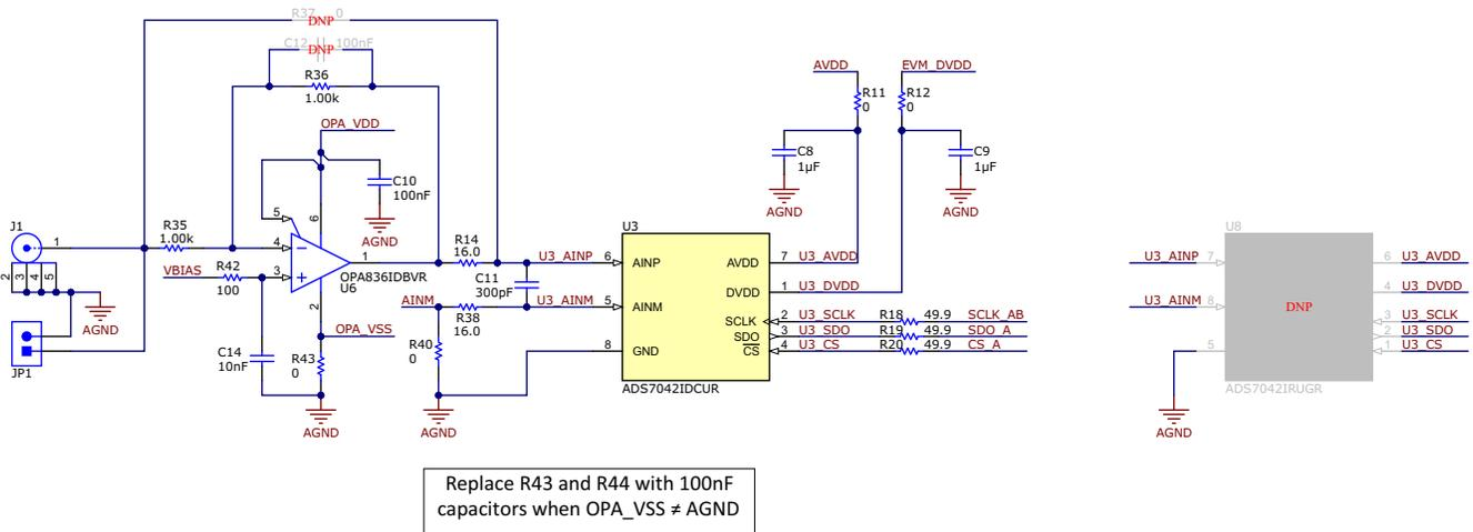
Figure 2-2. Single-Ended Input Path on the ADS704X-5XEVM
