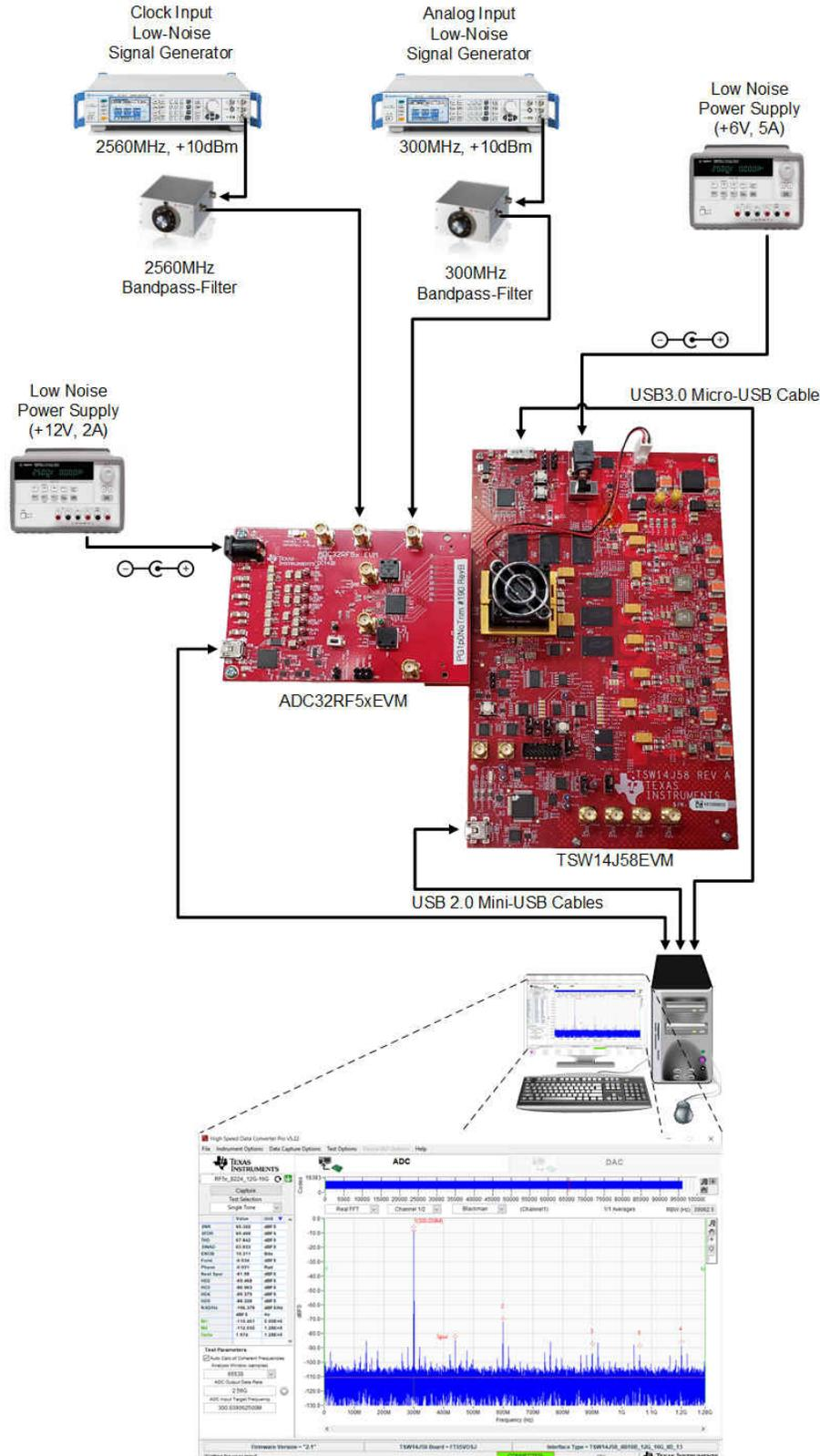
Figure 2-1. ADC32RF5xEVM Bench Setup Block Diagram
